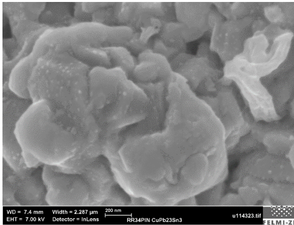
Figure 115 – CuPb23Sn3 (RR34). This image shows bright small dots at the structure surface. It was recorded at 7 keV and with InLens detector.
