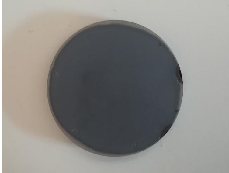
Figure 32 - A graduated layer system deposited on a M42 steel slice (top view on graduated layer).
