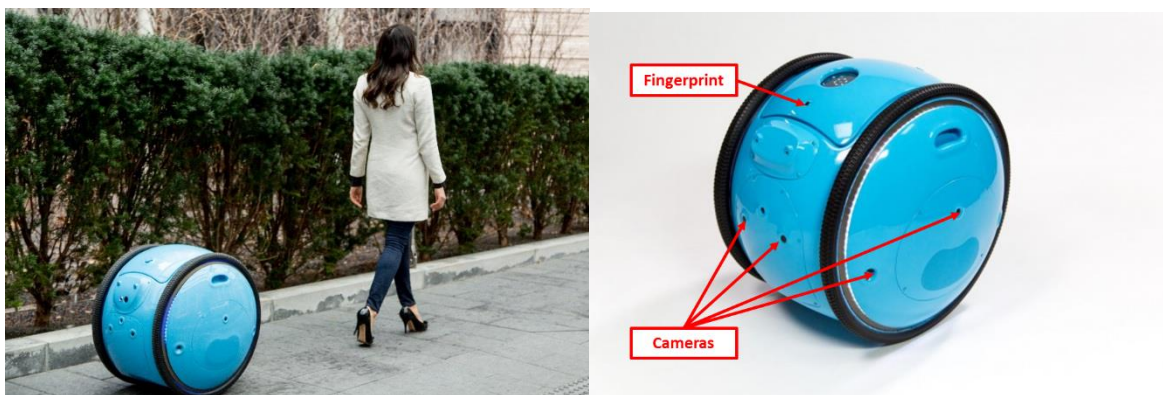
Figure 1.36 Autonomous luggage case Gita (64) and implemented sensor technologies (65)
