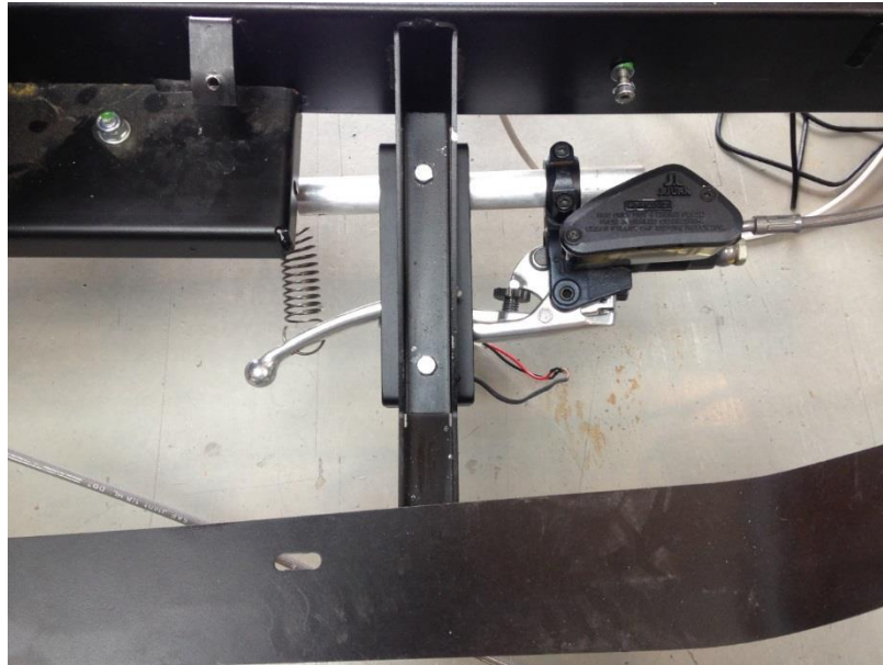
Figure 2.26 Emergency stop brake view 1
