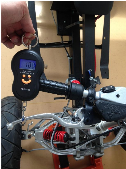
Figure 2.15 Force measurement on the brake lever at standstill
