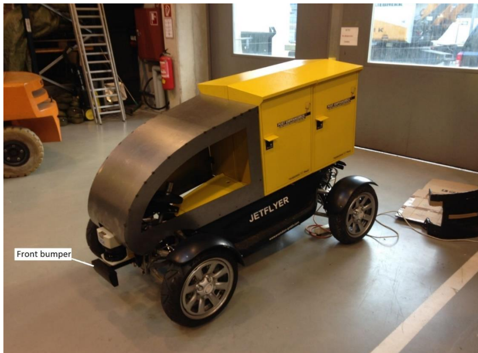
Figure 2.36 Adapted front fairing on the Jetflyer
