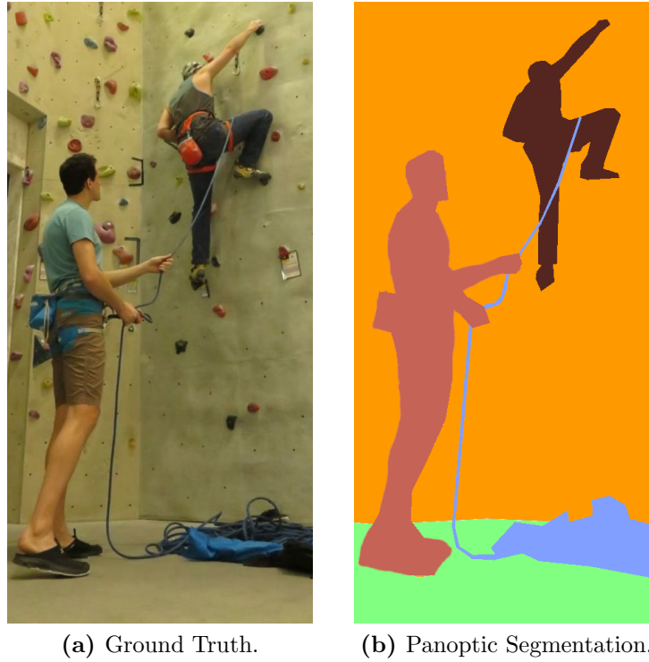
Figure 2.25: An example of panoptic segmentation. Each pixel is associated with a class label. Additionally, instances belonging to the same class are separated.
