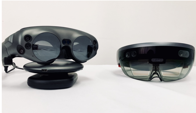
Figure 2.5: Comparison of AR HMDs: Magic Leap (left) next to Microsoft HoloLens (right), reprinted from 4Experience (2019).
