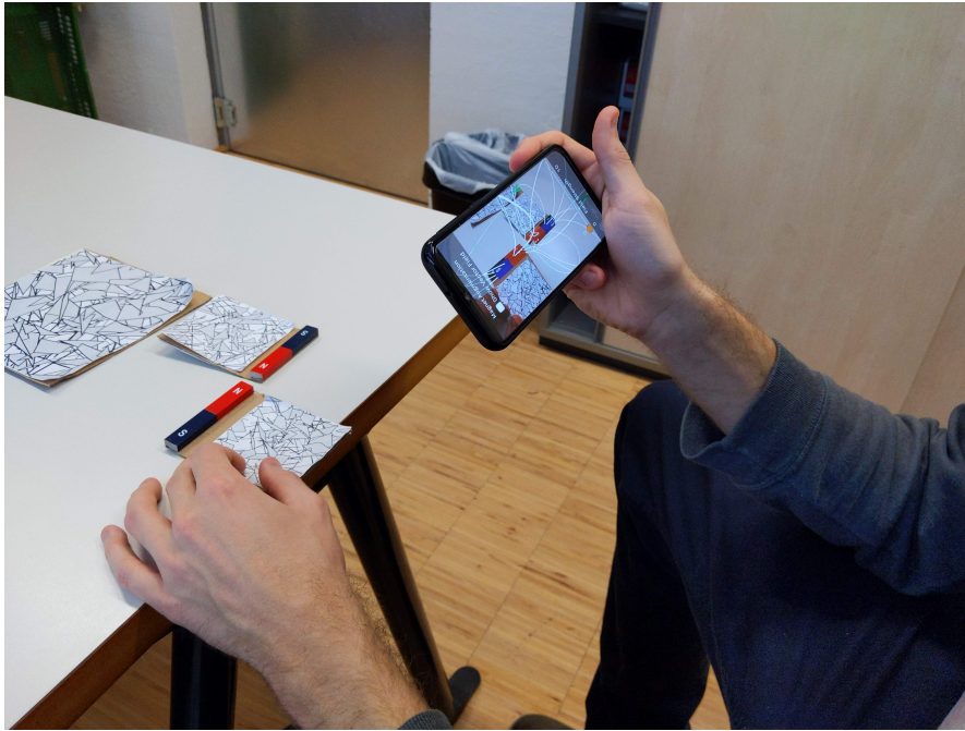
Figure 5.2: The test setup for the mobile AR application, showing a study participant pointing the smartphone at two real magnets which are tracked by the attached custom-printed image targets.
