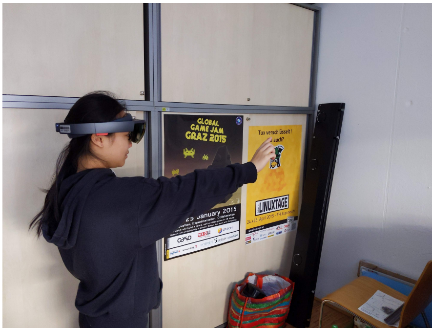
Figure 5.1: The test setup for the HoloLens AR application, showing a study participant performing a gesture while viewing the holographic content which is anchored on the white wall space in front of her.
