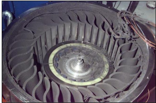
Figure 9: Dropped and crashed rotor from Boeing [10]
