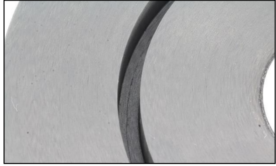
Figure 74: Circular crack on the groove bottom
