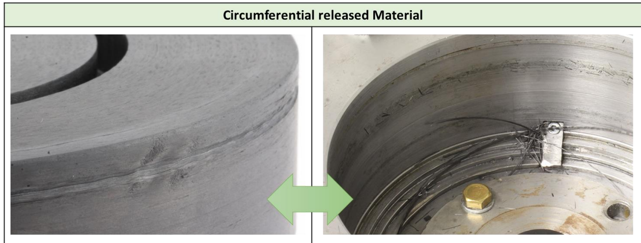
Figure 75: Rotor damage due to released circumferential material (left) and remaining debris after the test (right)
