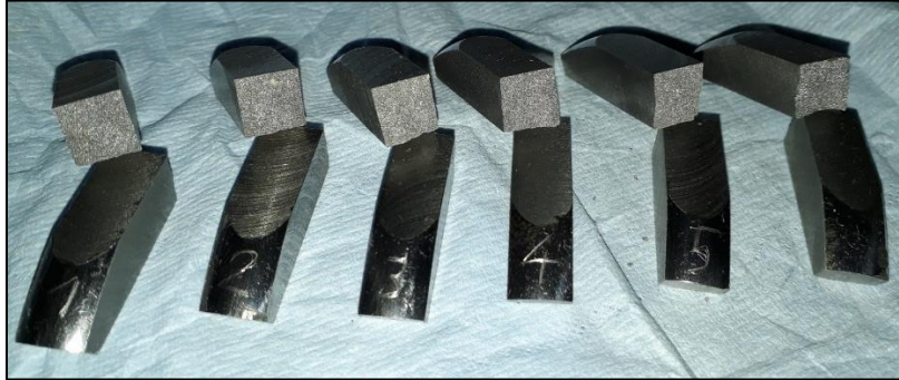
Figure 34: Samples of cast iron handwheel material prepared for a notch bar test
