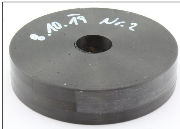
Figure 49: Cured and turned CFRP burst rotor
