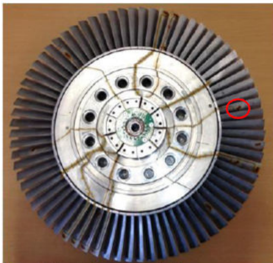
Figure 2 Rotor strain gauge application
