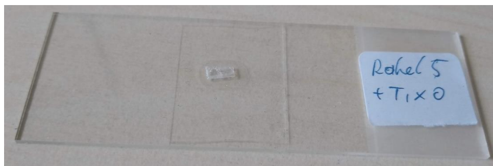
Figure 5.3: Customary adhesive tape applied on a glass substrate to hold the sample PMLF in place.
