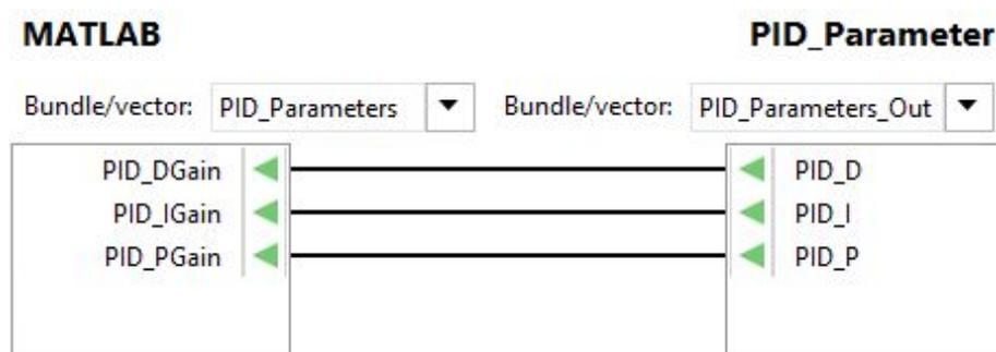
Figure 2.3: Example of ports connection inside the bundles
