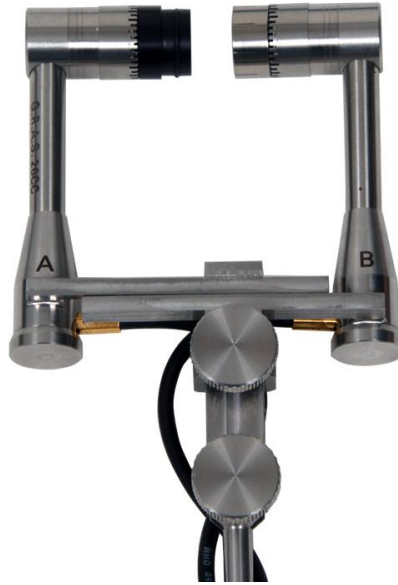
Figure 1-2: Sound intensity probe with two microphones [3]
