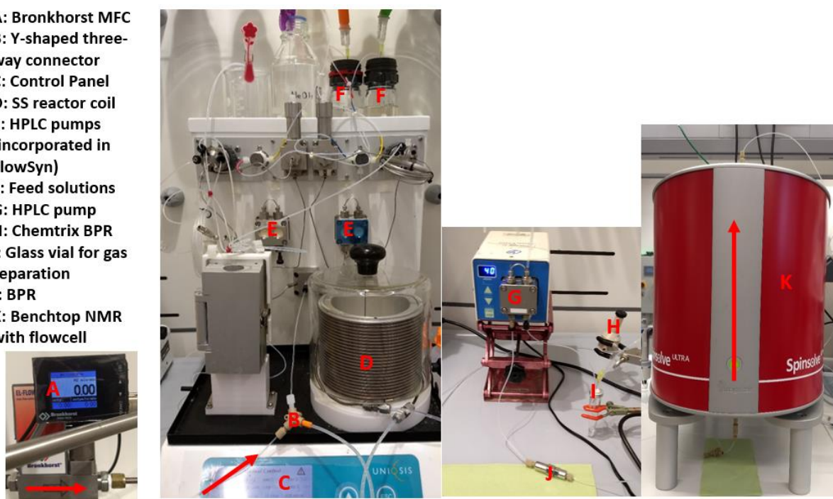
Figure 5.4.2: Labelled flow setup for the long run of the Ru-MACHO hydrogenation.
