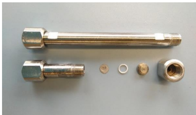
Figure 15. HPLC column-L: L x I.D. 120 x 8 mm (top); HPLC column-S: L x I.D. 40 x 8 mm (bottom left); filter, sealing ring, sealing cap, column cap (bottom right)
