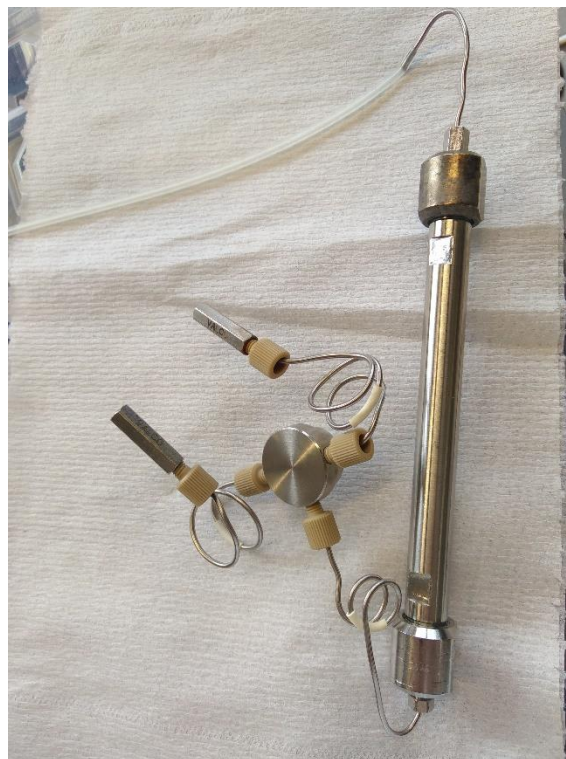
Figure A 3. Packed column-L for Heck reactions in combined setups (experiment B2 and B3) with T-mixer
