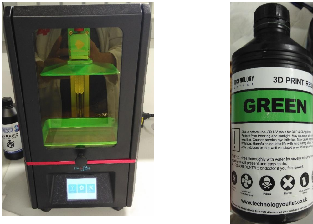
Figure 17. left: Anycubic Photon 3D-printer; right: Technology Outlet 3D print resin (green)
