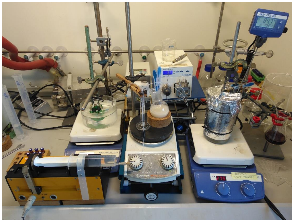
Figure A 5. Combined reaction setup of experiment B3. Decarboxylation in CSTR and Heck coupling in column-L
