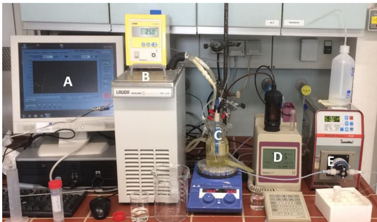
Figure 14: General set-up for the preparative scale production of C12-OHs with the P450 BM3/GDH reaction system. (A) PC monitoring O 2 concentration, (B) Brinkmann Lauda Ecoline RE104 Recirculating chiller for temperature control, (C) Double-walled reaction vessel (Wheaton) containing pH electrode and titration tip, O 2 sensor and O 2 inflow and standing on a magnetic stirrer plate, (D) TitroLine Alpha titration device for pH stabilization, (E) MCP-CPG piston pump used for fed-batch supplementation of C12:0.
