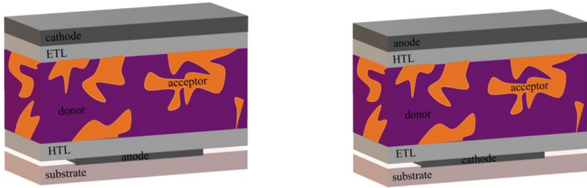
Figure 3: Bulk-heterojunction solar cell in normal (left) and inverted (right) device architecture.
