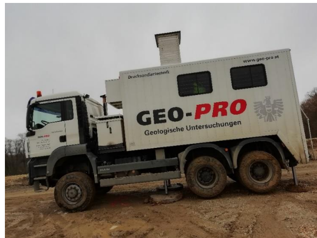
Fig. 3: Heavy-duty truck for in-situ testing from Geo-Pro
