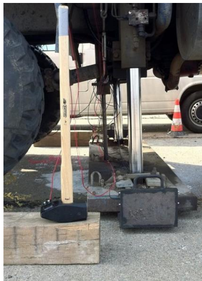
Fig. 6: Hammer and steel beam for seismic test (geotechnik, 2013)
