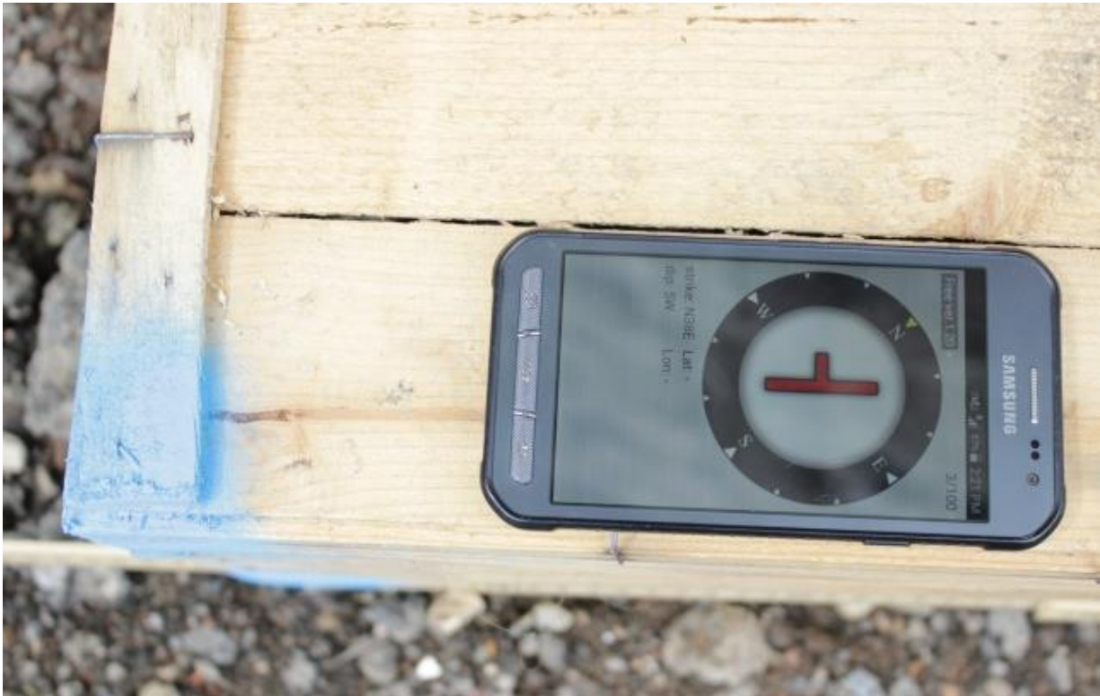
Figure 15: Measurement of the Orientation using the app geoClino
