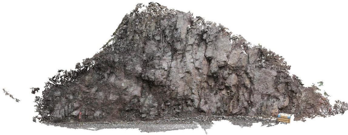
Figure 44: Point cloud of the outcrop, on the bottom right the box used for geo-referencing is clearly visible
