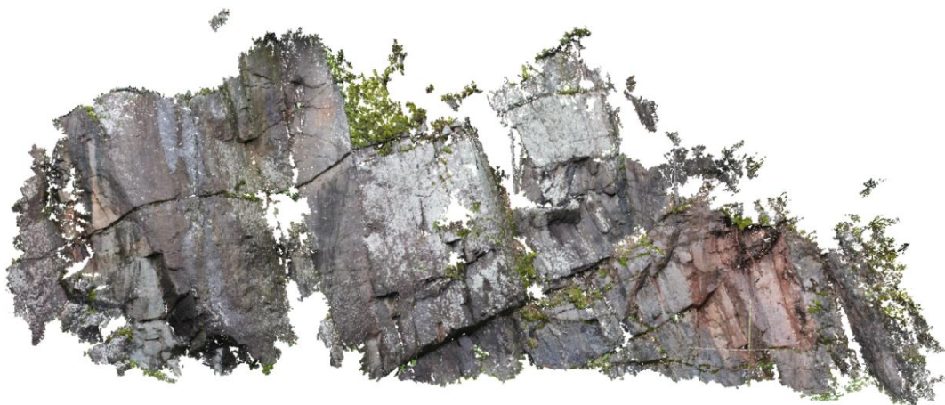
Figure 24: Dense point cloud of the outcrop, the white patches is areas where vegetation covers the rock surface. On the bottom right a fresh breakout is clearly visible (reddish colour) that also follows the same joints as the other surfaces
