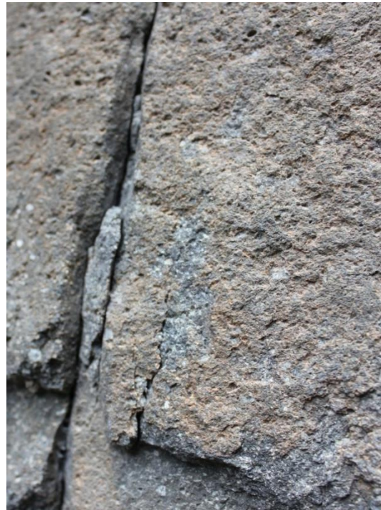
Figure 3: Left; close up view of the mineral structure of the rhyodacitic rocks, with the clearly visible “salami” structure caused by the amorphous rock mass with small phenocrystals (whitedots) Right; slightly altered surface next to a discontinuity.
