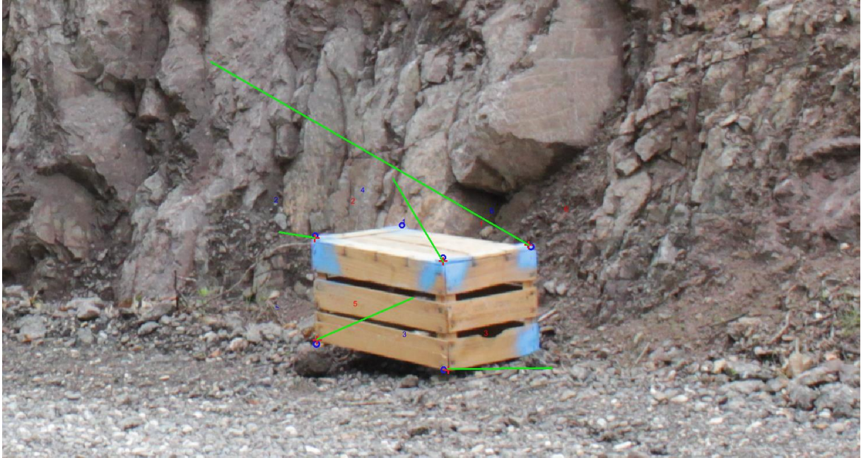
Figure 13: Example of Ground control points matching, using SfM_georef. The red crosses are the manually selected GCPs inside the picture; the blue circles indicate the position of the GCPs after the transformation; the green lines indicate the shift of each control point.
