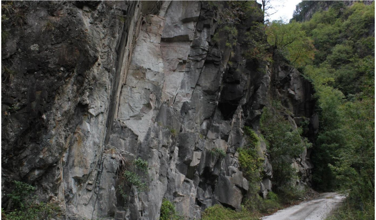
Figure 29: Overview of the outcrop. The picture is taken parallel to the subvertical discontinuities of the set 1, showing well their orientation and persistence through the rock mass.
