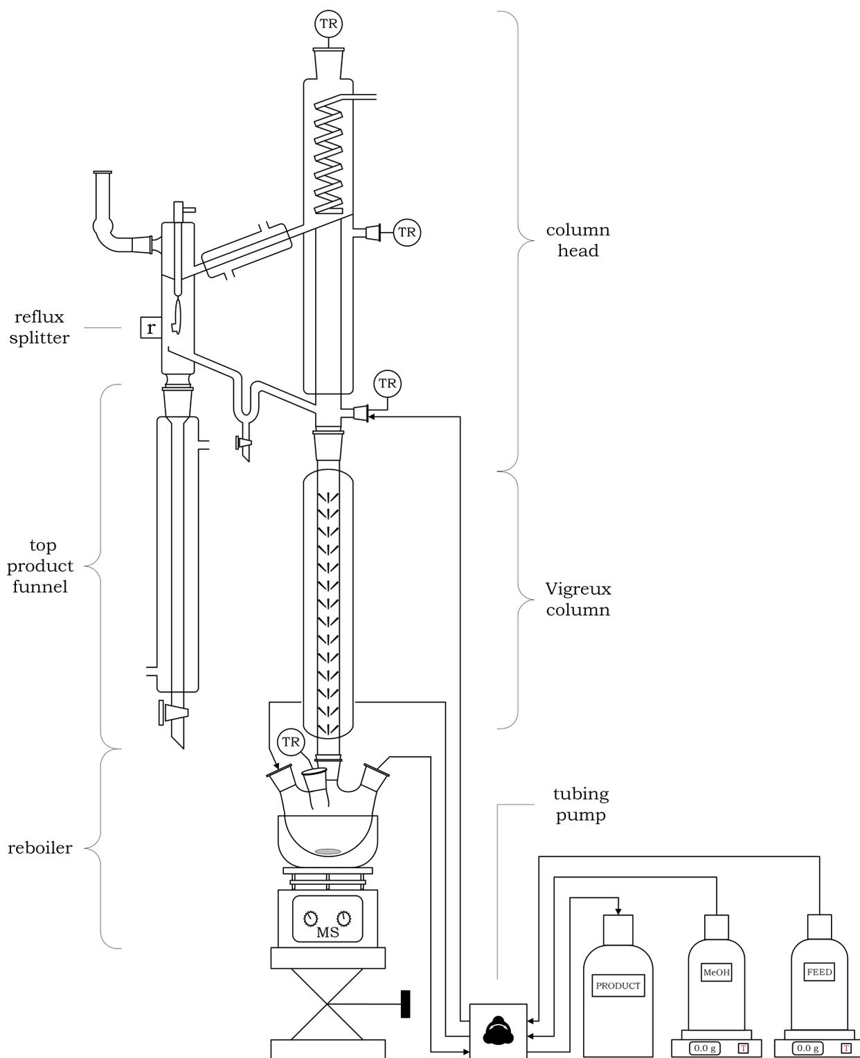
**Figure 8.2.:** Schema of the (dis-)continuous benchtop reactive distillation setup with a 500 ml four-neck flask as reboiler, a 30 cm Vigreux column and a three-channel peristaltic pump.
