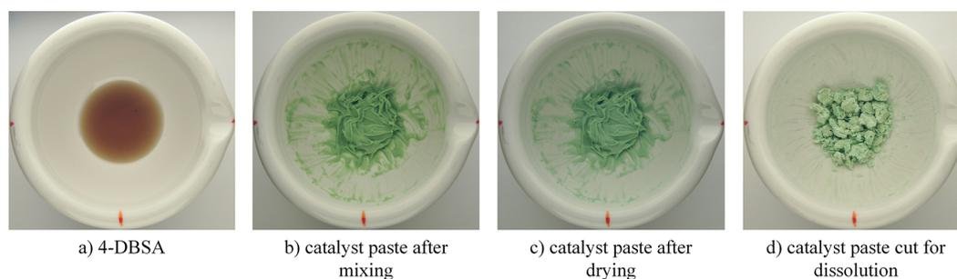
**Figure 1.** Preparation steps of the nickel-metallosurfactant catalyst  $\text{Ni}(\text{DBSA})_2$ : (a) 4-DBSA before admixture of  $\text{Ni}(\text{OH})_2$ ; (b) catalyst paste right after mixing of 4-DBSA and  $\text{Ni}(\text{OH})_2$ ; (c) catalyst paste after 3 days storage at ambient conditions; and (d) cut catalyst paste prepared for dissolution in the solvent phase.
