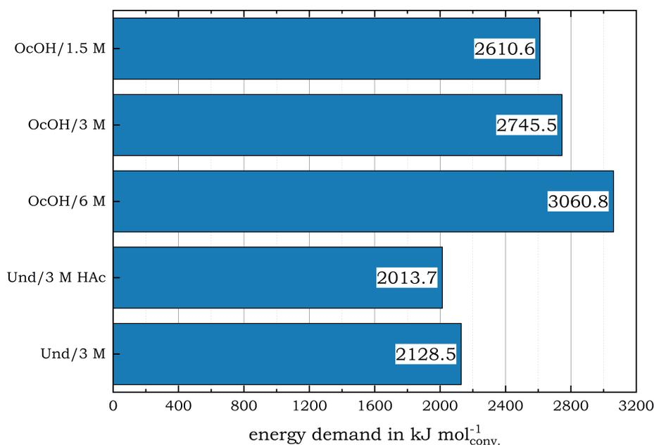
**Figure 8.12.:** Specific energy demand based on the amount of substance converted in steady-state; amount of substance converted: sum of converted octyl acetate and acetic acid.
