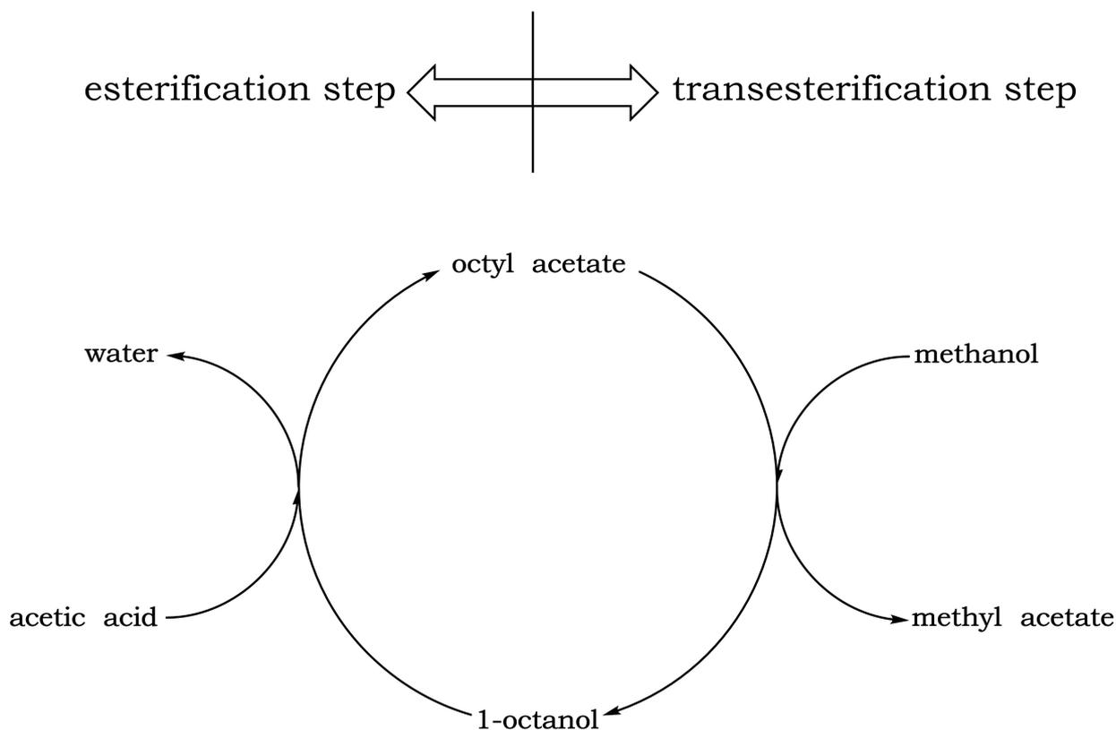
**Figure 9.1.:** Reaction cycle of low-molecular-weight carboxylic acid and 1-octanol in the proposed reactive separation process concept, exemplarily shown for acetic acid; esterification step: acetic acid is esterified with 1-octanol to water and octyl acetate; transesterification step: octyl acetate is transesterified with methanol to methyl acetate and 1-octanol.
