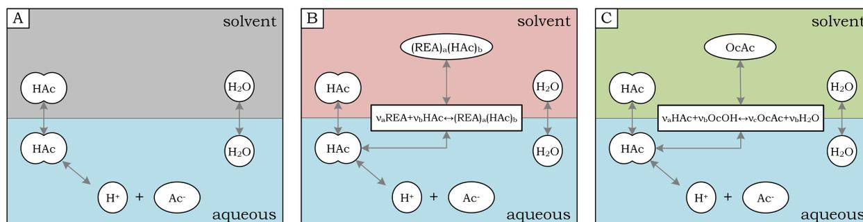
**Figure 4.4.:** Principle schemes of liquid-liquid extraction types. A: physical extraction. B: reactive extraction *via* adduct formation. C: reactive extraction *via* chemical conversion.
