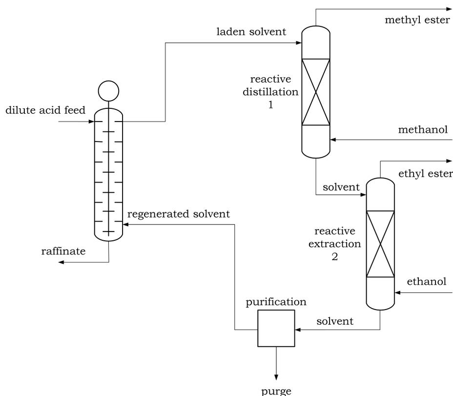
**Figure 4.6.:** Solvent regeneration *via* reactive distillation in a reactive extraction process as patented by Tirronen et al. [62]. Reactive extractant agent: Cyanex<sup>®</sup>923.
