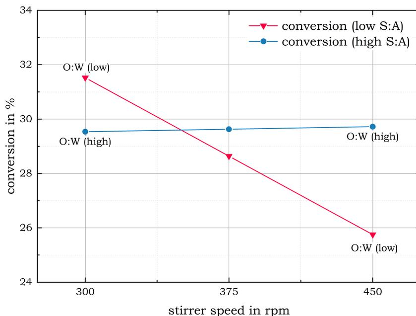
**Figure 4.3.:** Interaction plot as a tool for evaluation of parameter interaction in DoE. Interaction of solvent to aqueous ratio (S:A) and stirrer speed and its impact on conversion in reactive liquid-liquid extraction in emulsion as described in Chapter 6.
