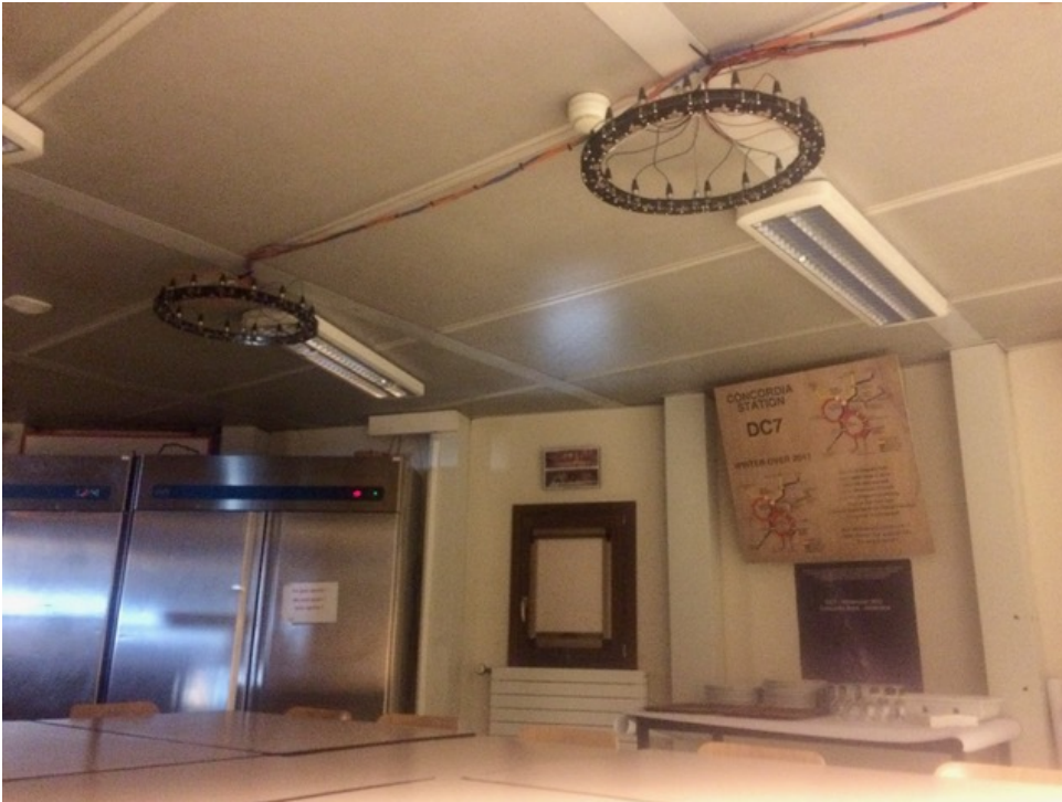
Figure 1.2: Microphone arrays mounted above the dinner table
