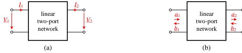
Figure 2.1.1: (a) General two-port network with currents and voltages and (b) the equivalent power waves [32].
