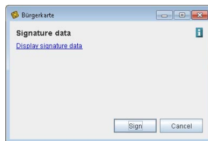
Fig. 3. The GUI of MOCCA Local allows users to review data to be signed and to start the signature creation process
