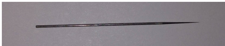
Figure 38: Tungsten tip, which has to be re-sharpened.
