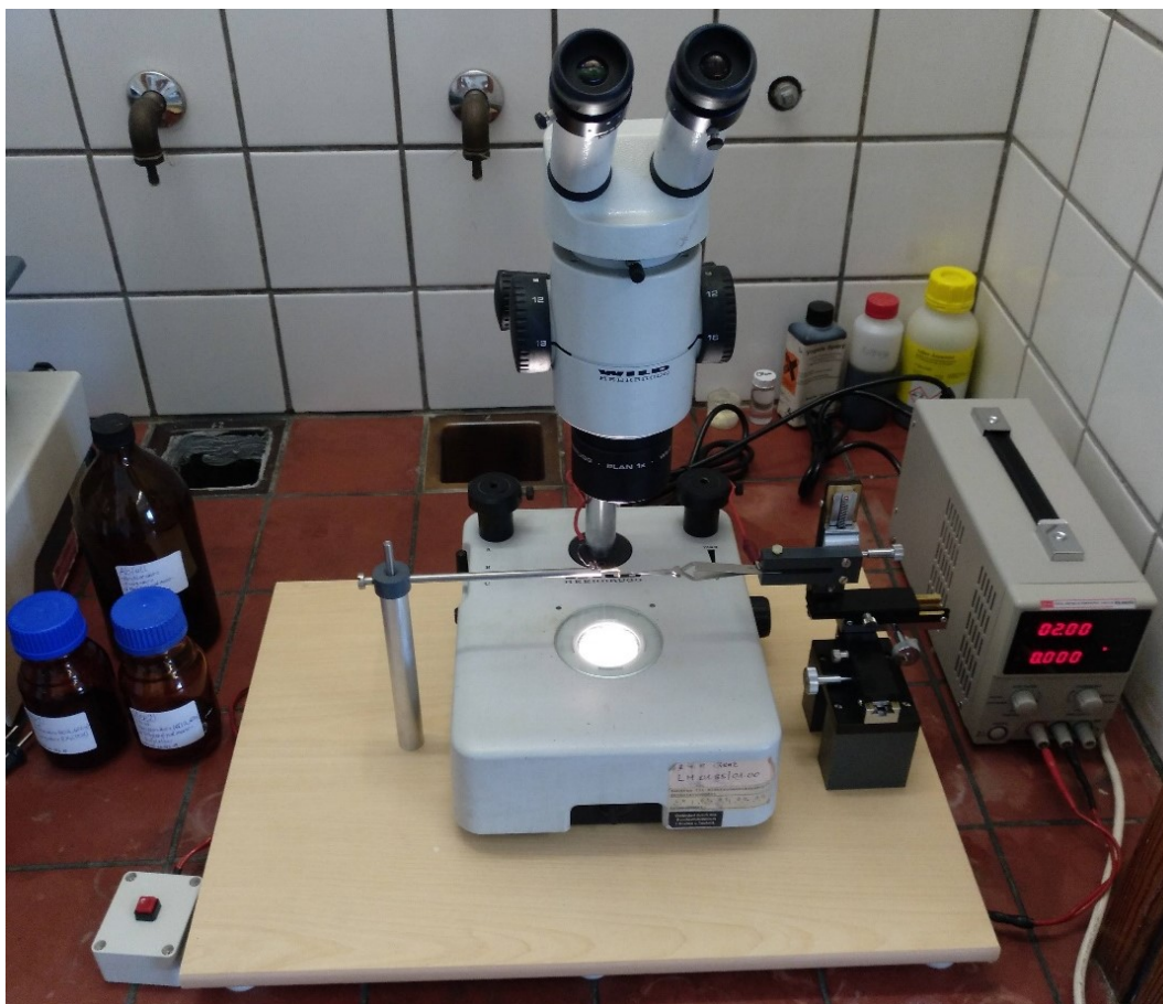
Figure 20: Overview of the realized apparatus for the nanotip preparation.
