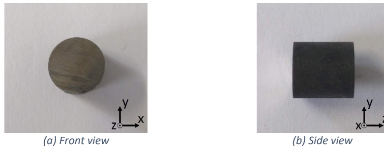
Figure 31: Starting material of the Inconel 718 alloy. A cylinder with a diameter of 1 cm and length of around 1 cm.
