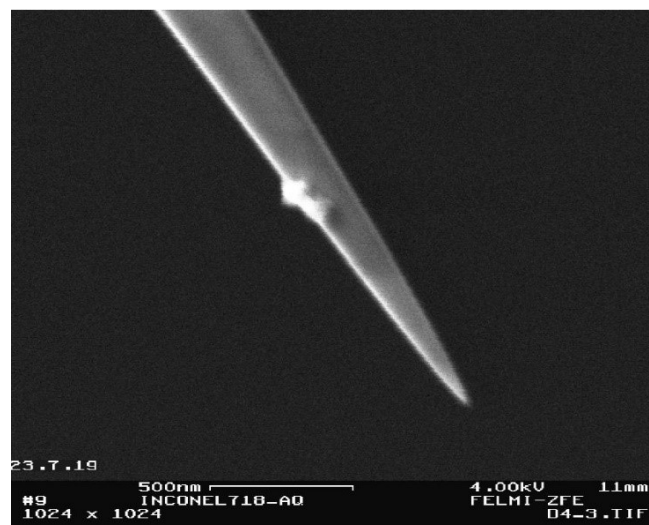
Figure 23: Example for the demonstration of the evaluation of nanotips. This is the original image, which is loaded into the script for further calculations.
