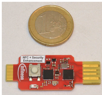
Figure 6.9: NFC + Security enhancement evaluation stick.
