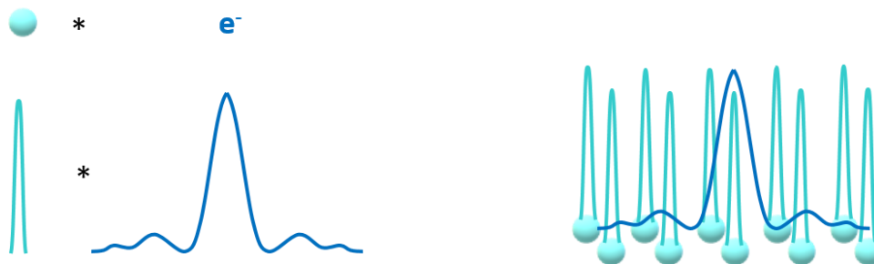
Figure 7: Scheme of convolution of object function and probe intensity profile delivering HAADF image intensity.
