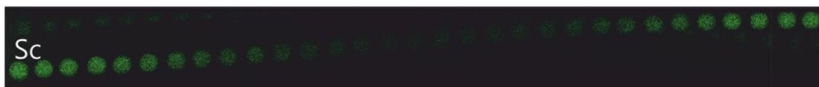
Figure 31: Horizontally stitched EDX elemental map from stitched SI resulting from SI tilt series. All spectrum images acquired throughout the tilt series are horizontally aligned next to each other to form one large SI that can be processed at once. The variation of intensities throughout the tilt series stems from shadowing of the EDX detectors and is discussed in section 5.1.1
