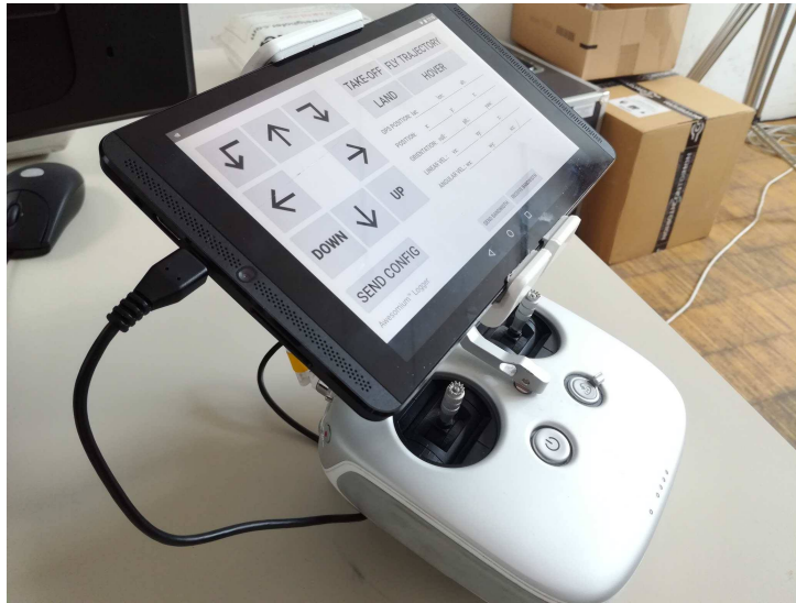
Figure 2.2: An image showing the RC connected to the tablet via a USB cable. On the screen we can see our demo application for MAVLink communication.
