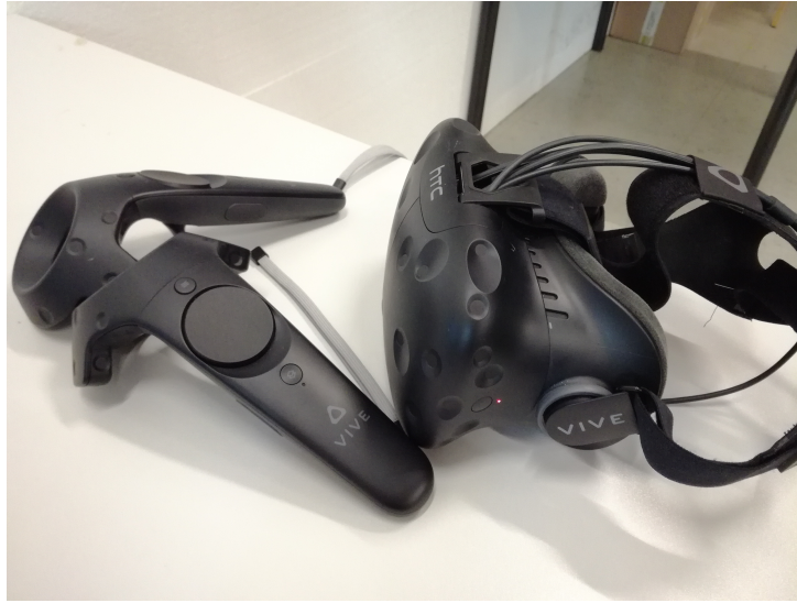
Figure 2.3: An image of the HTC Vive headset and controllers used during the project.
