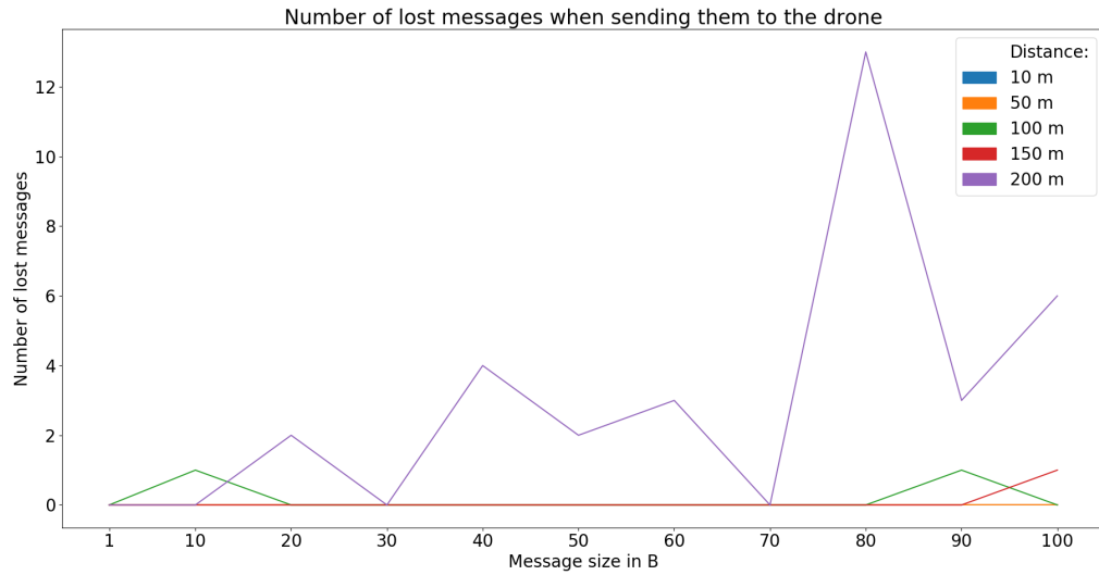
Figure 3.7: A graph of the number of messages lost out of 100, when sent from the Android application to the ROS node on the drone.
