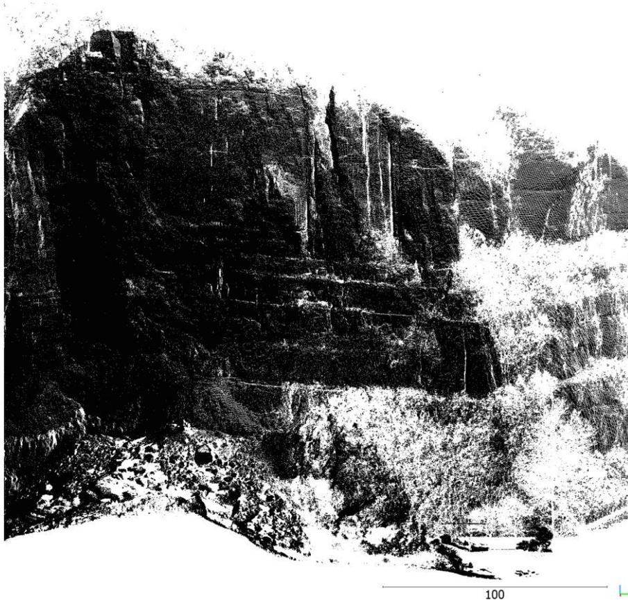
figure 5: This unprocessed point cloud of the outcrop Long Chang shows the variability in point density, dependent on the surface orientation. Horizontal and vertical traces with low densities, perpendicular to the overall face orientation are witnessed. A combination of line of sight bias and resolution bias could lead to a neglect of these sets.
