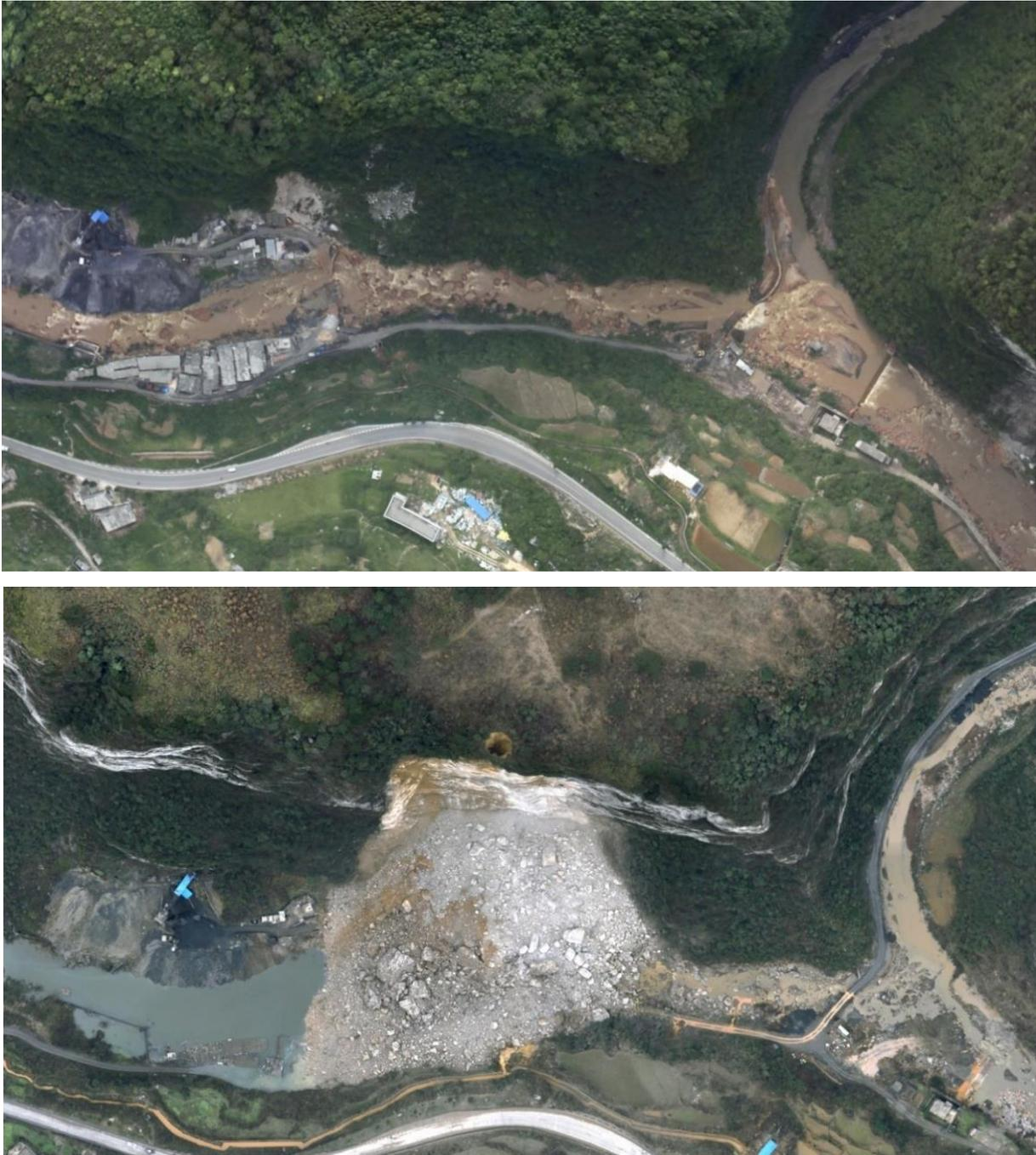
figure 2: The two aerial photos show the outcrop Long Chang. The upper photo was taken before, the lower photo after the rock fall event. The sinkhole in the upper middle of the lower photo is clearly visible and indicates high karst activity.
