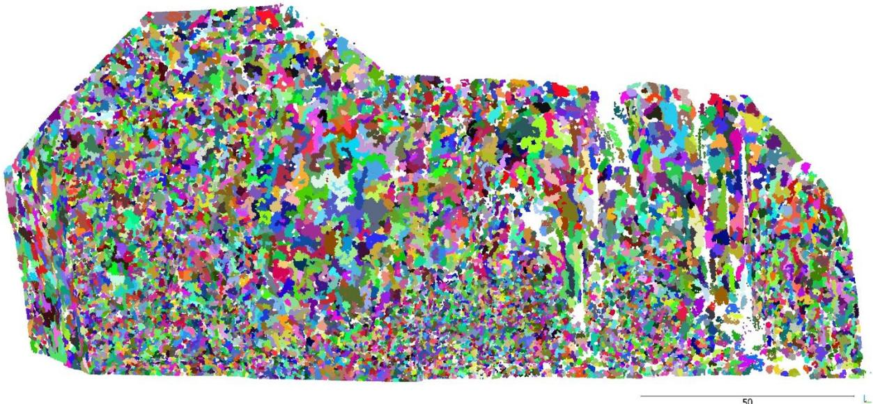
figure 21: In the plane model of the semi-automatic methodology for Long Chang each plane, which fulfils the planarity conditions, is displayed in one colour.
