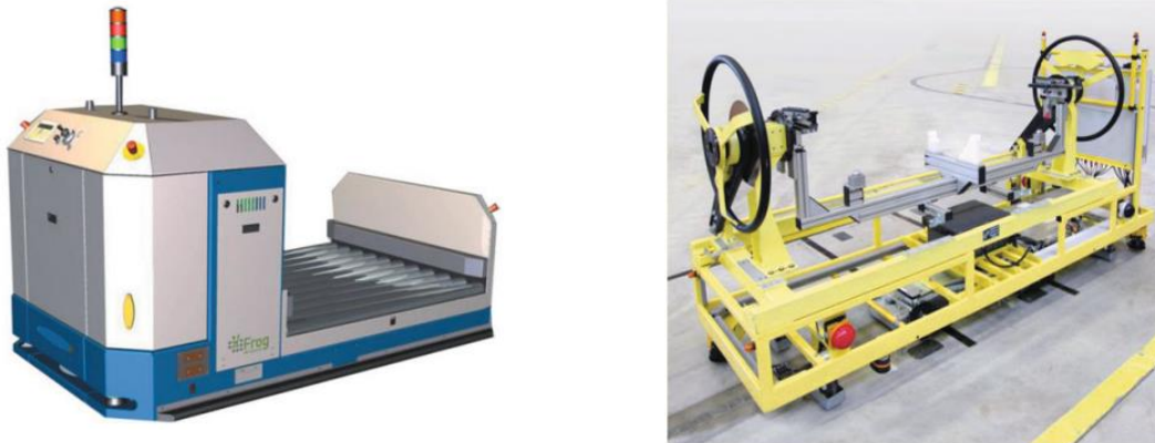
Figure 27: (a) Piggyback AGV (b) Assembly AGV. Source: Ullrich (2015).
