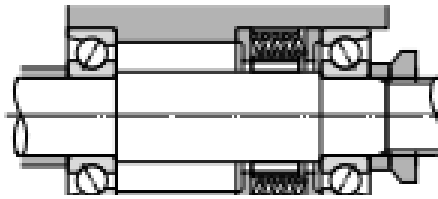
Figure 11: Extract preloading using spring. Source: NTN (2015).
