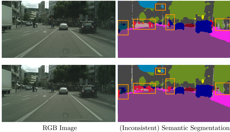
Figure 1.2: Inconsistent Semantic Segmentation. The state-of-the-art algorithm [66] has problems keeping a consistent view of the street scene. A few significant differences are highlighted by orange boxes.
