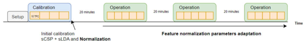
Figure 3.6: The simulation scenario of the AdLDA algorithm. sCSP and sLDA were calibrated with normalized features after the calibration block and were used in the operation blocks with the adaptation of normalization parameters.
