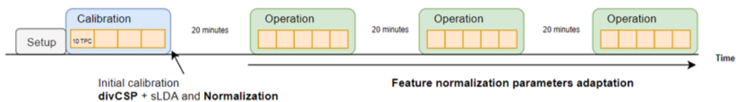
Figure 3.9: The simulation scenario of AdLDA + divCSP-WS . The calibration was done with divCSP-WS , sLDA, and features normalization. In the operation blocks, the normalization parameters were adapted.
