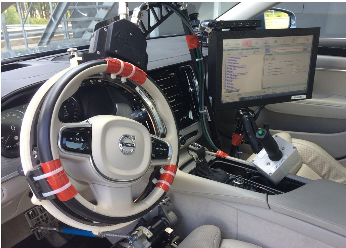
*Figure 8.9: Steering robot used for executing driving trajectories.*
