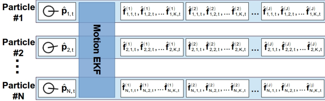
Figure 4.4: Representation of the individual particles in the extended FastSLAM algorithm.
