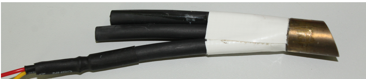
Figure 4.17: The phototransistor is connected to the bundle by means of a heat shrink tube. Due to the opaque tube, ambient light does not have any impact on the connection.
