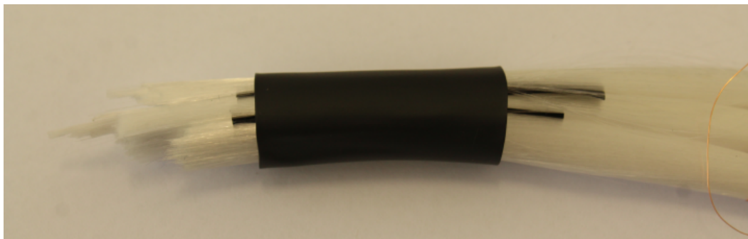
Figure 4.5: The heat shrink tube compresses the bundles. It helps to achieve the desired shape of the sensor surface.
