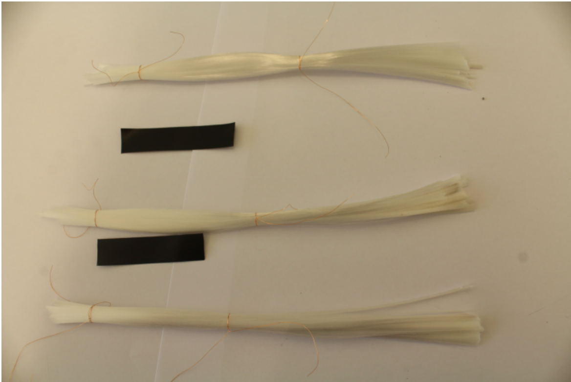
Figure 4.3: Premerging of the fibres to form the bundles. A black electrical tape separates the bundles.
