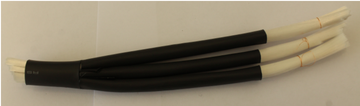
Figure 4.6: The separation and compression of the single bundles is done by means of heat shrink tubes. These are opaque and attached to the first tube as close as possible to minimize any influence of ambient light.
