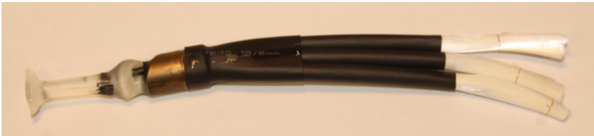
Figure 4.9: After the cure the funnel is removed and the transparent adhesive can be seen. The sensor head is now completely sealed, and the sheath is mounted to the main tube and the bundles.
