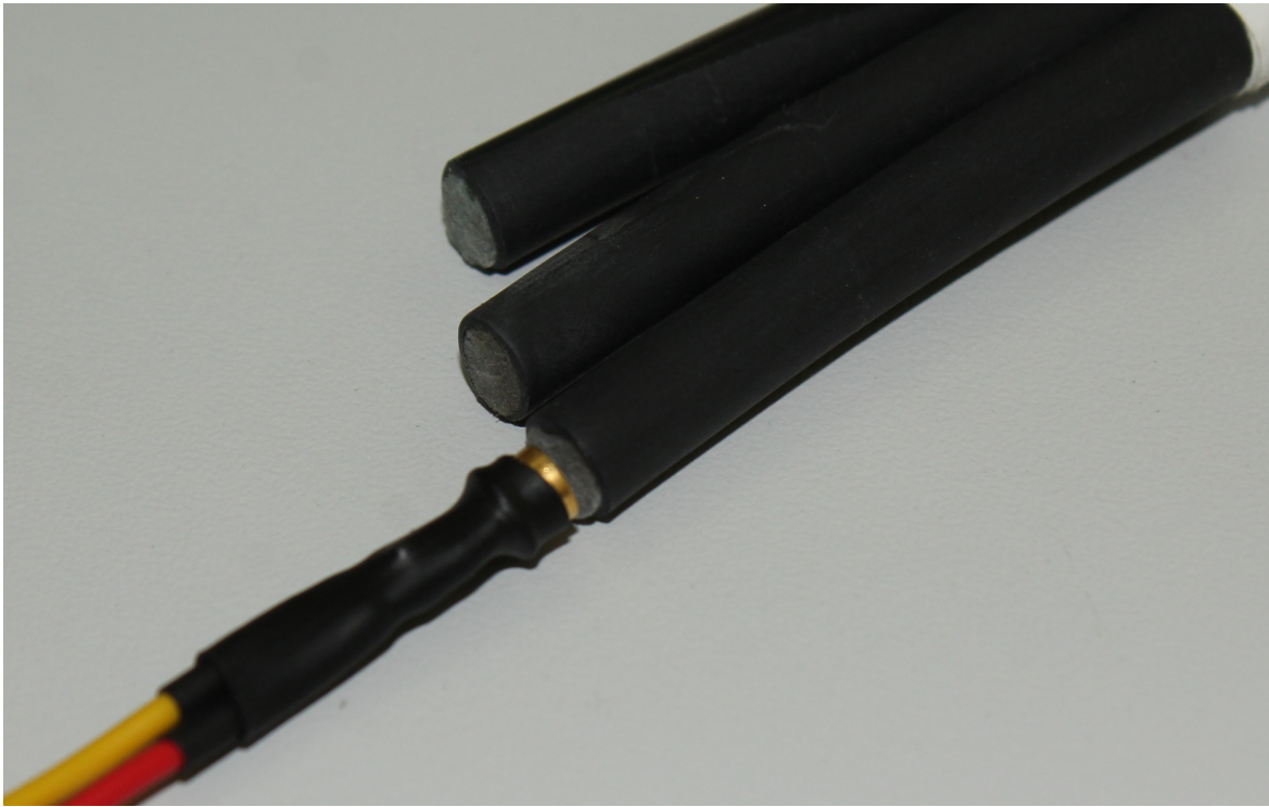
Figure 4.16: The phototransistors are placed as close as possible to the corresponding signal bundles to ensure a suitable optical transmission.
