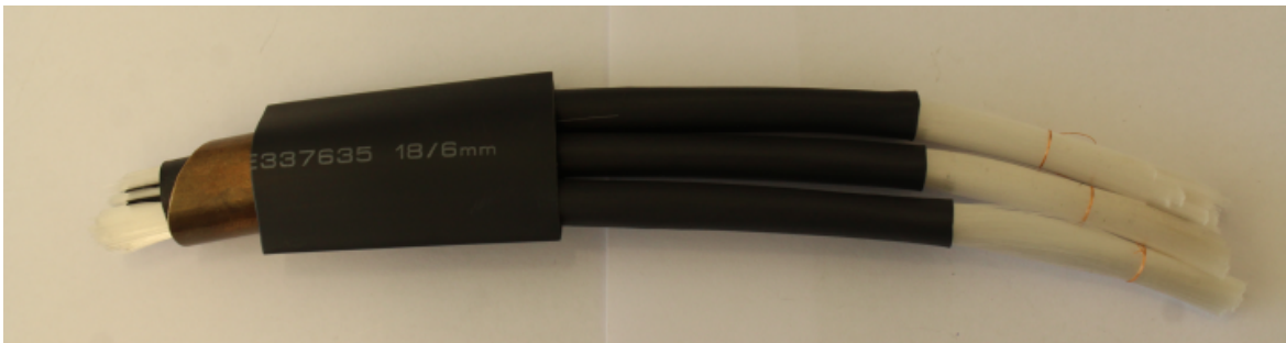
Figure 4.7: A metallic sheath covers the main tube and the inner fibre structure. A further heat shrink tube is used to hold the sheath in its desired position.
