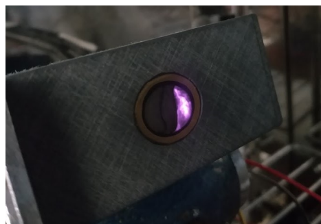
Figure 4.23: Complete illumination of the source bundle at lowered ambient light.
