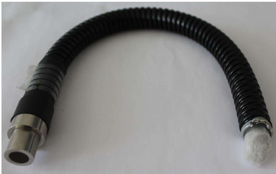
Figure 4.1: Raw material for the construction of the sensor. The fibres are extracted from the coating and cut to a suitable length for the sensor.
