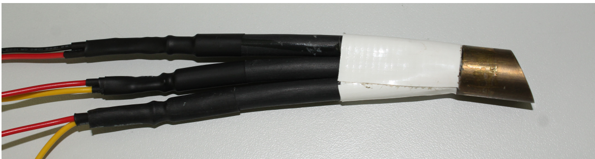
Figure 4.20: Sensor with connected LED and phototransistors. The electronic components are coupled to the bundles using heat shrink tubes. An opaque adhesive is used to shield the area between the metallic sheath and the single bundles from ambient light.
