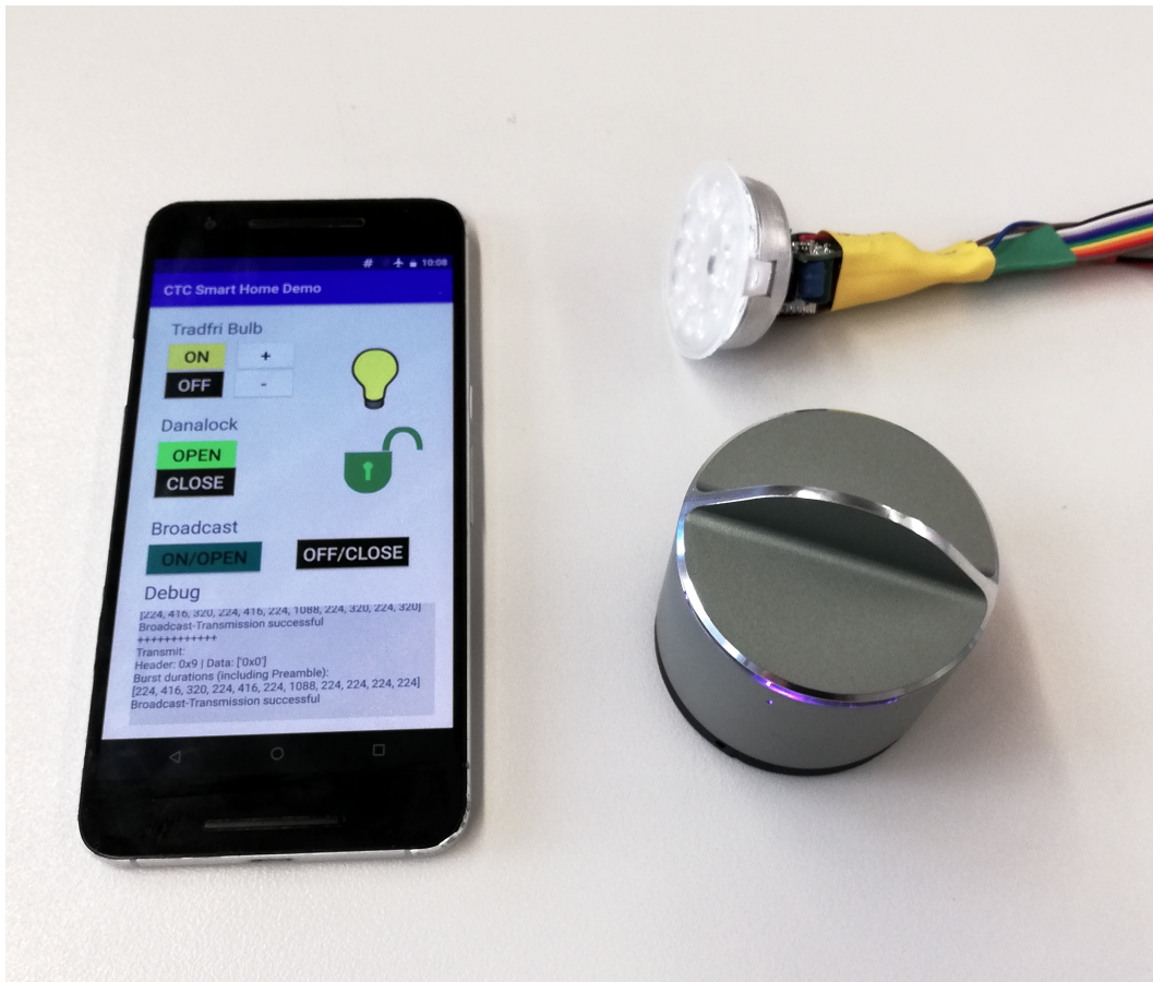
Figure 6.13: Devices used in the CTC smart home demonstrator: a Nexus 6P smartphone, an IKEA Trådfri light bulb and a Danalock V3 door lock.
