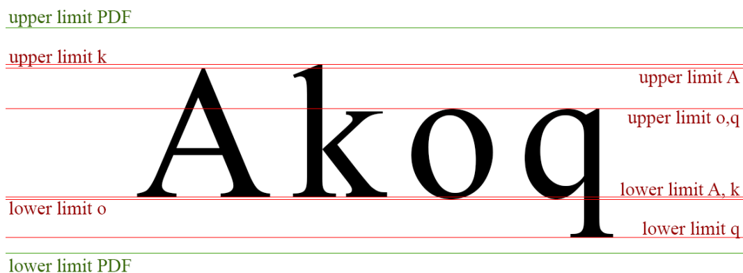
Figure 3.4: Four letters in the same font and font size start and end at different y-coordinates. The PDF bounding boxes around these letters have the same y-coordinates (green lines). However, the PDF coordinates are much larger than the actual characters (red lines).
