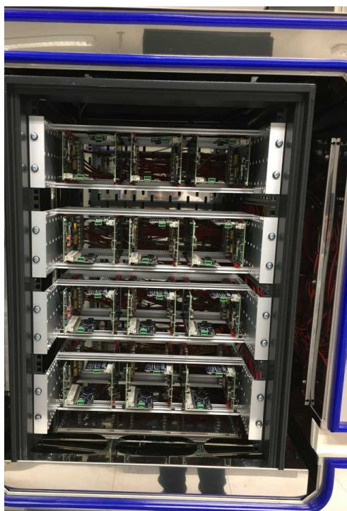
Figure 3.2: Climate chamber that exerts stress on semiconductor power devices.
