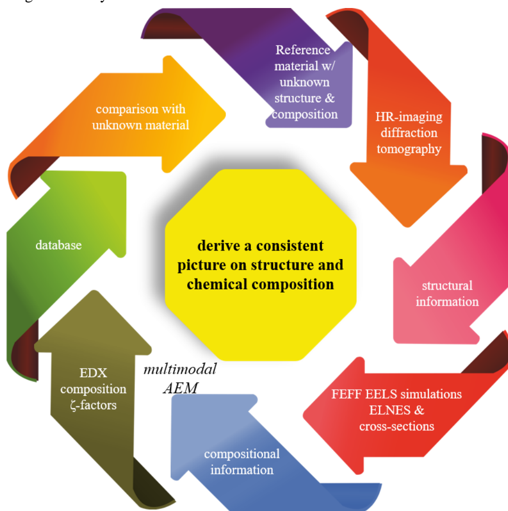
Fig. 46 Characterization path envisioning the combination of structural as well as analytical TEM methods to gain a consistent picture on the crystallographic structure and chemical composition of materials.
