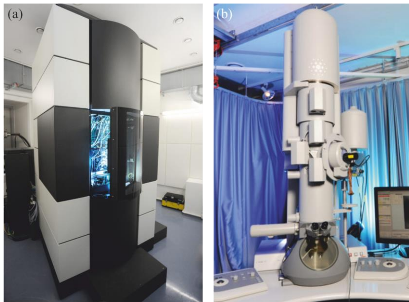
Fig. 8 Electron microscopes mainly used within this work at the FELMI-ZFE in Graz: (a) FEI TITAN 3 , (b) FEI Tecnai 200.
