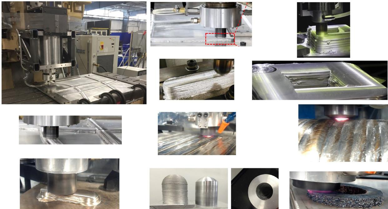
Fig. 3.7: Types of structures successfully deposited by MELD [25].
