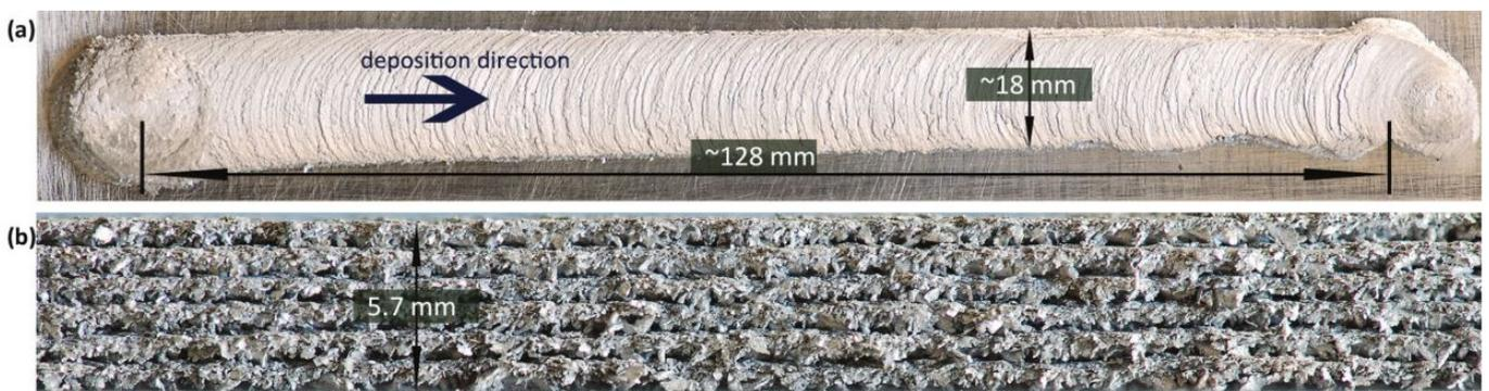
Fig. 3.6: Multi layer deposition of AA5083 on a AA2024 substrate produced with the FS process: (a) top view, (b) side view with the individual layers [23].
