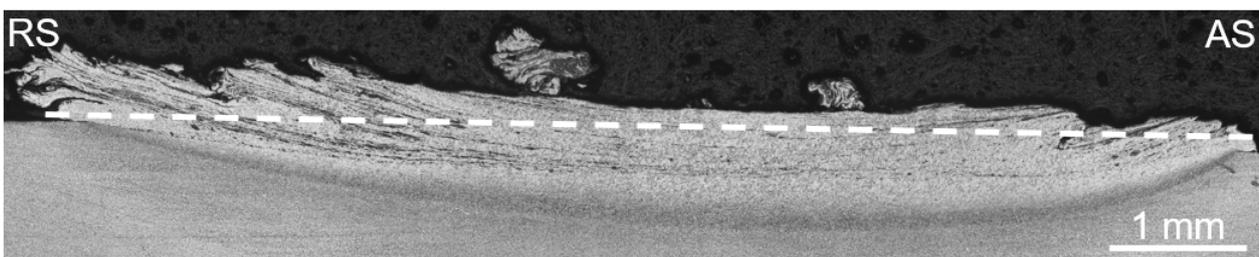
Fig. 5.8: Position of the hardness line on an 8 mm rod deposition.
