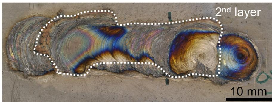
Fig. 5.24: Example of a double-layer achieved with a 12 mm rod (2<sup>nd</sup> layer in the white dotted line). 1<sup>st</sup> layer: 3200 min<sup>-1</sup>, 0.5 kN, 700 mm/min; 2<sup>nd</sup> layer: same as 1<sup>st</sup> layer but displacement of the shortening stage was altered to 1.5 mm.
