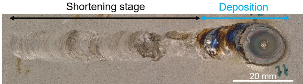
Fig. 5.10: Impact of insufficient energy input during the shortening stage on the layer quality; 0.7 kN shortening force and 1.0 mm displacement.
