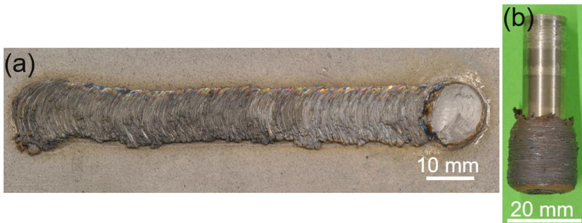
Fig. 5.11: (a) Deposition with a 12 mm rod and (b) corresponding flash;  $3000 \text{ min}^{-1}$ , 0.5 kN, 800 mm/min.
