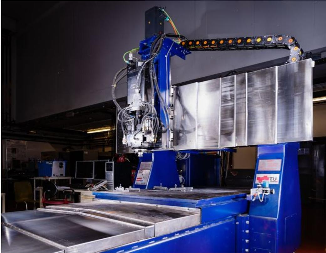
Fig. 4.1: MTS Friction stir welding machine used in this work.
