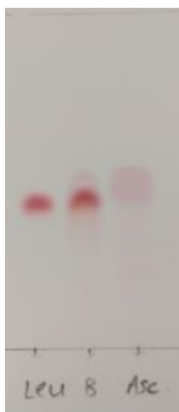
Figure 42: Identification of ascorbate as reaction component visible in all samples of the blank reaction. [Leu] Leucine standard 5 mM; [B] Blank reaction at t_1 ; [Asc] Ascorbate 10 mM.
