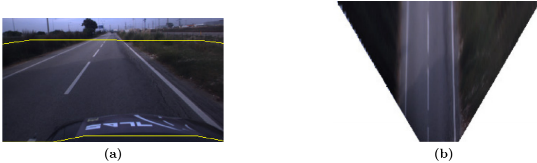
Figure 3.3: Inverse perspective mapping with a) as input image and b) as the bird-eye image. The yellow line indicates the area of the image that was used for IPM . Image taken from [43].
