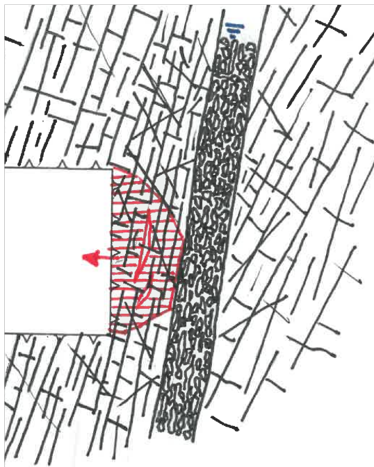
a) Plug failure / cracking
