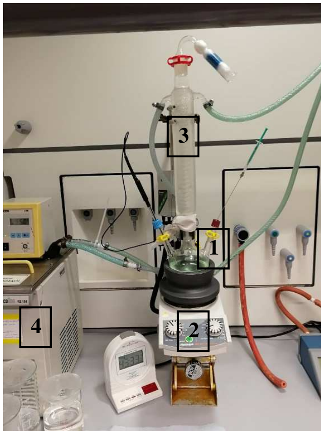
Figure 9: Experimental setup for kinetic batch experiments in lab scale for kinetic experiments with round-bottom flask (1), heating stirrer (2), cooler (3) and thermostat (4)
