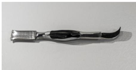
**Figure 3.13:** LIG-PDMS rolled supercapacitor device with one terminal covered with Al contact
