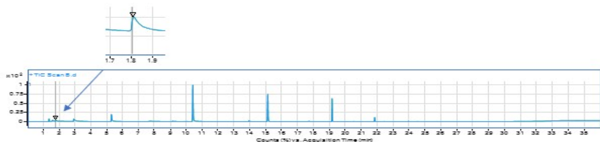
Figure 66: Chromatogram of uninoculated BBM media produced at the institute of environmental biotechnology at TU Graz. Enhanced image of peak detection indicated by the blue arrow.
