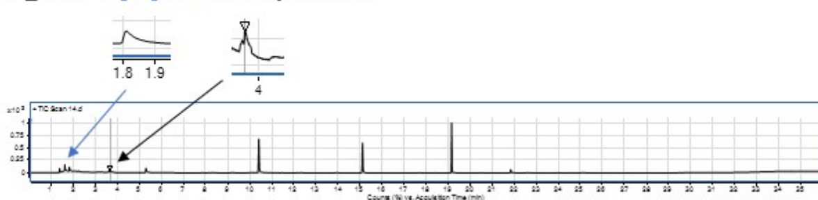
Figure 62: Chromatogram of H. pluvialis strain HP_G01. Enhanced image of peak detection indicated by blue and black arrows.
