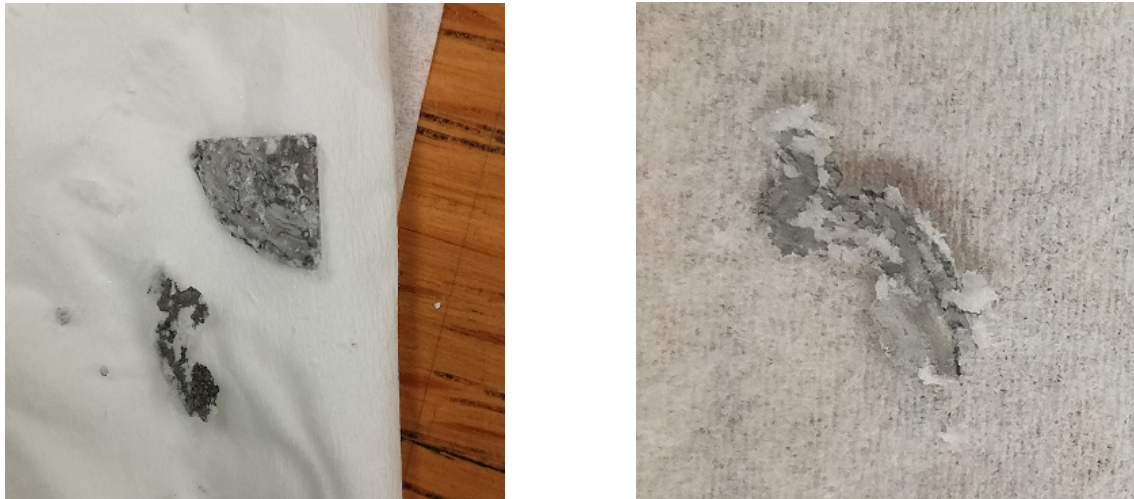
Figure 32: Photograph of a detached surface patch of the HPT-deformed Mg-alloy after 24 h of in-vitro corrosion in SBF (radius of the sample ca. 7.5 mm). Left: Patch as detached from the surface. Right: Corrosion products formed underneath the detached patch.
