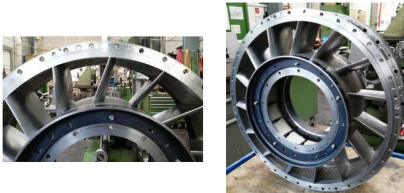
Figure 4.15: Leaned TEC with soft end walls
