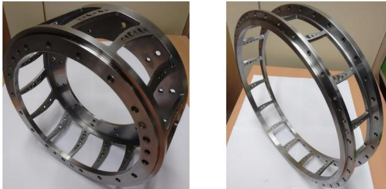
Figure 4.12: Inner (left) and outer (right) ring of the resonator TEC
