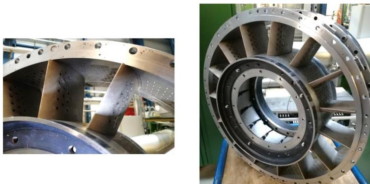
Figure 4.16: Helmholtz vanes with soft end walls
