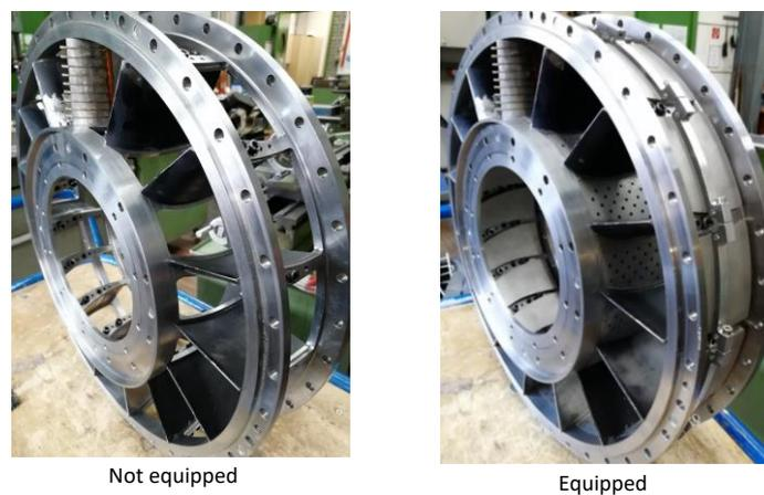
Figure 4.13: Standard TEC with and without soft end walls
