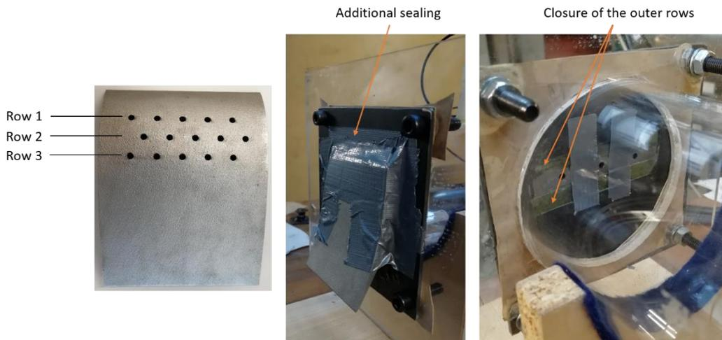
Figure 6.1: Vane mount at the impedance tube
