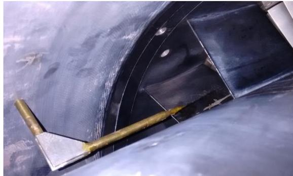
Figure 5.8: Trailing edge probe inside the test rig
