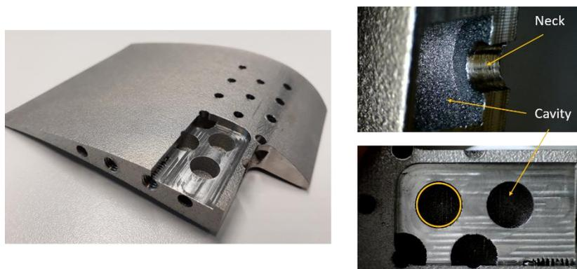
Figure 4.3: Cut of a Helmholtz vane
