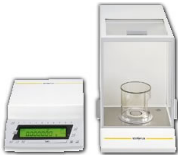
Figure 17: Fine scale used for weighting the samples: Sartorius model MC21S
