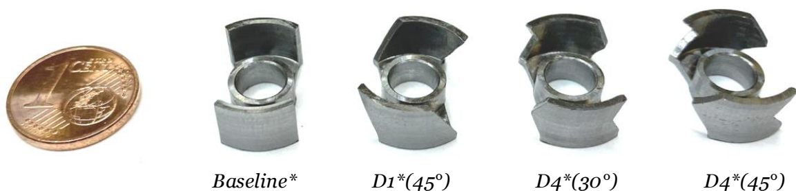
Fig. 8.6: Prototype stator parts milled from free-cutting steel 11SMnPb37 to investigate Design 4 and Design 5 .
