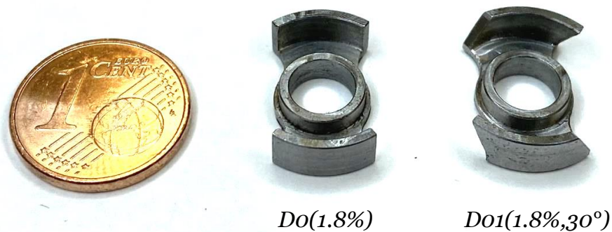
Fig. 6.4: Prototype stator parts milled from free-cutting steel 11SMnPb37 to investigate Design 1 .
