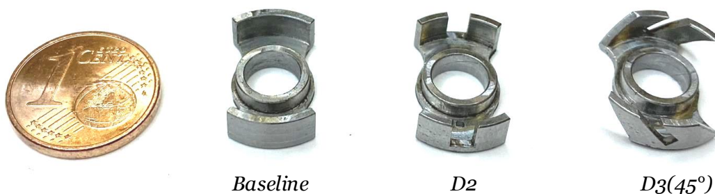
Fig. 7.6: Prototype stator parts milled from free-cutting steel 11SMnPb37 to investigate Design 2 and Design 3 .
