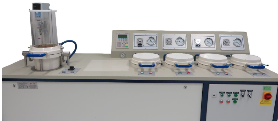
Figure 3.4 Rapid-Köthen Handsheet former equipped with a white water recirculation system [15]
