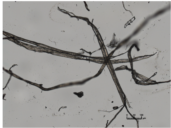
Figure 4.18 Microscopy image of reference pulp with fines
