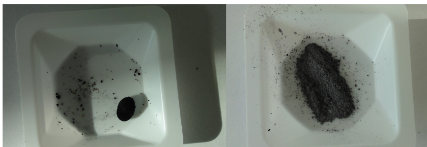
Figure 17.: image of NTiL pellet after solid state synthesis, T = 700\text{ }^\circ\text{C} , dwelling time = 15 h
