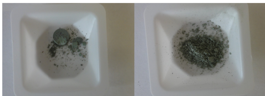
Figure 21.: image NCrL pellet after the solid state synthesis, T = 600\text{ }^{\circ}\text{C} , dwelling time = 15 h
