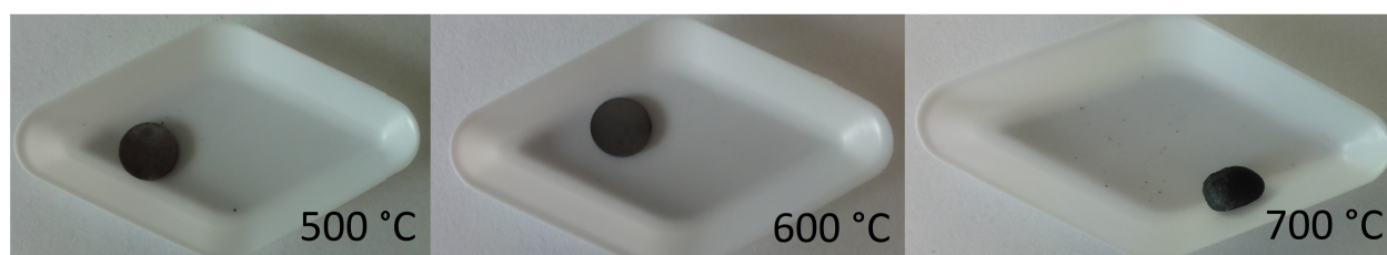
Figure 33.: image of samples with the chemical composition of NInL and dwelling time of 15 h, left sinter temperature 500 °C, middle sinter temperature 600 °C, right sinter temperature 700 °C [7]
