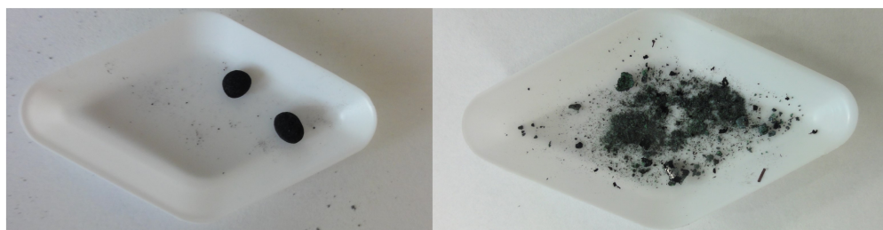
Figure 12.: image of sample after synthesis by Langley and Sturegeon, Left: NTiL sintered for 48 h at 850\text{ }^{\circ}\text{C} Right: NCrL sintered for 96 h at 900\text{ }^{\circ}\text{C}
