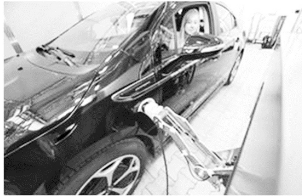
Figure 2.6.: Automated side coupler concept of the Technical University of Dortmund. The concept includes a special robot arm kinematic, which handles a standard charging plug, [DOR15].
