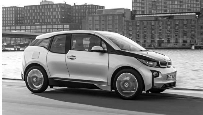
Figure A.1.: BMW i3 60 Ah, battery capacity 18.8 kWh, real range 130 km, energy consumption 14.5 kWh/100km, [DAT19]. The CCS Type 2 charging inlet of the vehicle serves as the main test object for ACCS prototype functionality. In addition, the vehicle was used for parking tests on the prototype charging lot.
