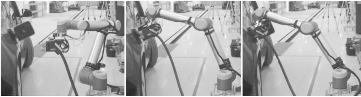
Figure 4.5.: Exemplary section of the charging connecting sequence. Left: Robot during inlet 3D-pose detection with Camera 3. Middle: CCS Type 2 connector axis aligns with the vehicle charging inlet axis. Right: Robot during the cable insertion process.
