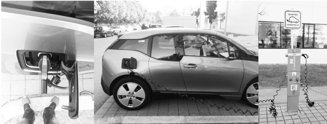
Figure 2.30.: Left: Side view of the EV with an open charging lid and plugged charging cable. Middle: Side view of the EV during battery charging. Right: 11 kW charging station with two Type 2 charging cables.
