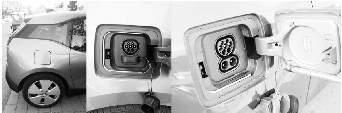
Figure 2.28.: Left: Side view of a BMW i3 with closed charging socket cover. Middle: View of the CCS Type 2 inlet with unplugged Type 2 inlet plastic flap. Right: View of final cover position and unplugged plastic flaps.
