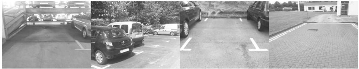
Figure 2.34.: Beginning from left, image 1, 2 and 3: Parking bays for testing the parking accuracy of test drivers. Image 4: Charging pad and parking conditions for testing the parking accuracy over a charging par without parking aids, [BWY + 15].
