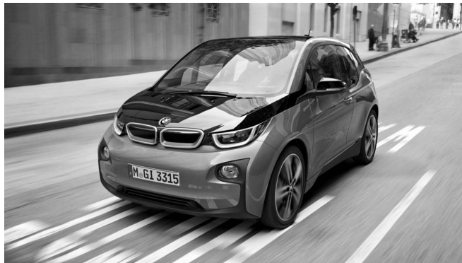
Figure A.2.: BMW i3 94 Ah, battery capacity 27.2 kWh, real range 170 km, energy consumption 16 kWh/100km, [DAT19]. The EV was used as 2 nd test object in the scenario of subsequently performed automated charging of different vehicles.
