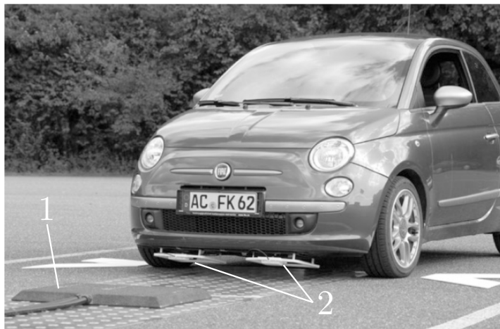
Figure 2.37.: Charging pad and positioning system of [BKHC15].
