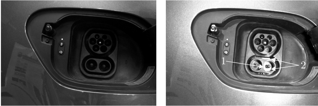
Figure 3.39.: Examples of inlet camera images without and with LED light support.
