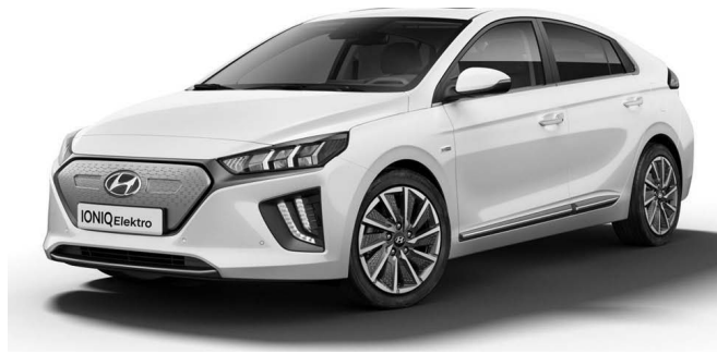
Figure A.4.: HYUNDAI IONIQ Elektro, battery capacity 38 kWh, WLTP range 294 km, energy consumption 13.8 kWh/100km, 0-100 km/h in 9.9 seconds, [HYU18a]. The vehicle served as the 5 rd ACCS prototype test EV.
