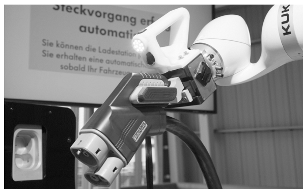
Figure 2.5.: ACCS concept with a KUKA robot arm, gripper and a CCS Type 2 connector, [VOL16].
