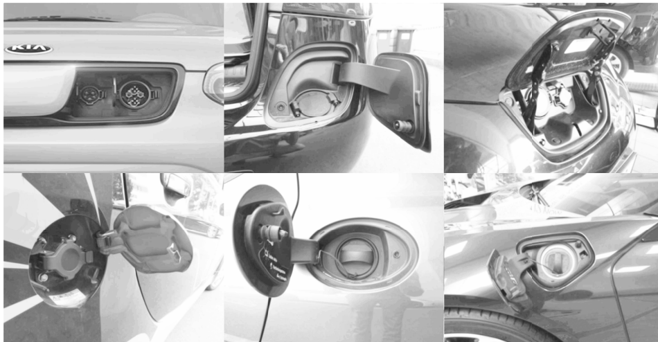
Figure 2.17.: Examples of various EV charging and security cap systems. Beginning from the top, left: KIA Soul EV (2015), MERCEDES C350 Hybrid (2015), NISSAN Leaf (2010), PEUGEOT iON (2011), PORSCHE Panamera S Hybrid (2013) and BMW i8 (2015).
