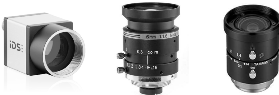
Figure 3.52.: Left: IDS 2D-Camera UI-5240CP-C-HQ Rev.2. Middle: Lens model LENSAGON C3M0616V2 1/1.8": 6 mm focal length, 60.1^\circ horizontal and 46.6^\circ vertical angle of view, [LEN19]. Right: Lens model TAMRON M118FM06 1/1.8": 6 mm focal length, 66.1^\circ horizontal and 50.8^\circ vertical angle of view, [TAM19].
