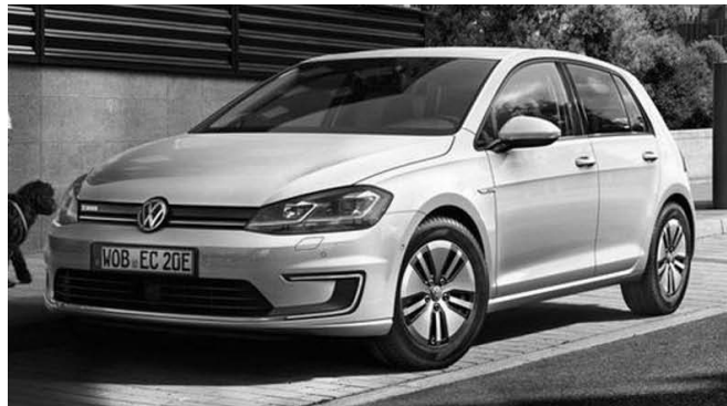
Figure A.5.: VOLKSWAGEN e-Golf, battery capacity 35.8 kWh, WLTP range 231 km, energy consumption 15.8 kWh/100km, [VOL18a]. The EV served as the 3 rd ACCS prototype test EV.
