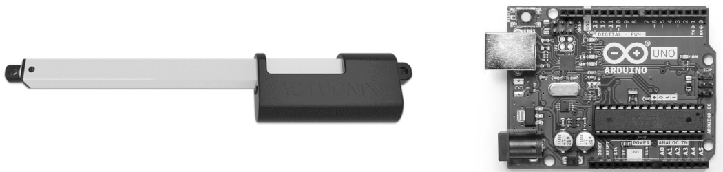
Figure 3.54.: Left: Linear actuator ACTUONIX P16-100-22-12-P, [ACT17]. Right: ARDUINO UNO REV3 microcontroller board, [ARD19].
