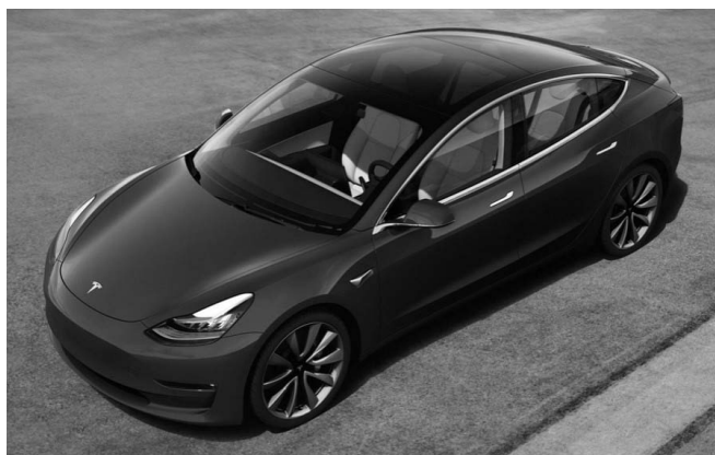
Figure A.3.: TESLA Model 3 standard version, battery capacity 53 kWh, WLTP range 409 km, energy consumption 14.1 kWh/100km, 0-100 km/h in 5.6 seconds, [TES20b]. The EV was the 4 th ACCS prototype test EV. The EV offers automated charging lid opening and closing.
