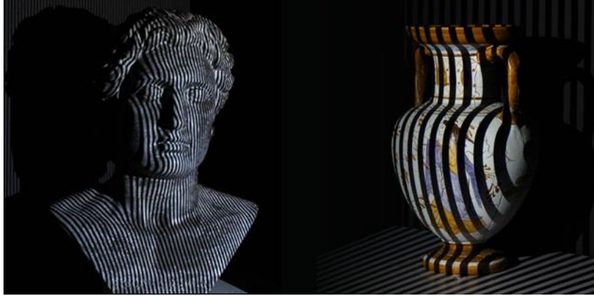
Figure 2.5: Distorted Structured Light [Kre16, Page 5]
