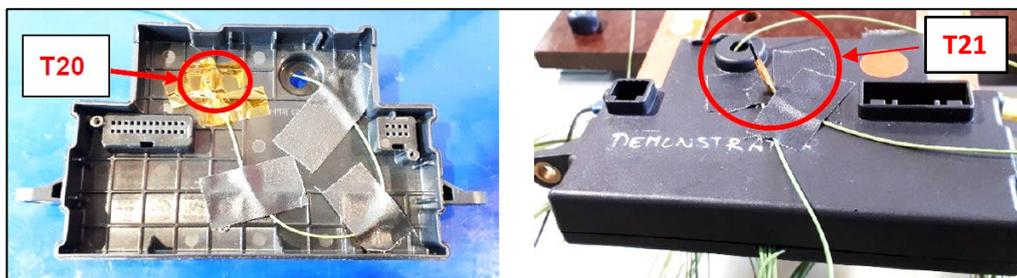
Figure 26: Thermocouple inside the BDU housing (on the left) and outside the BDU with 1 cm distance (on the right) [29]
