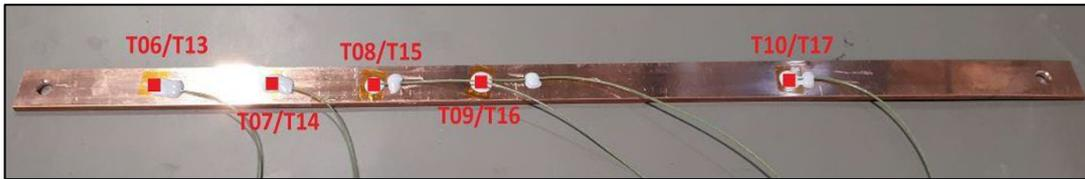
Figure 32: Busbar thermocouples position [29]
