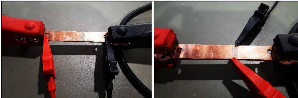
**Figure 27:** Shunt transition resistance measurement (on the left) and manganin transition resistance measurement (on the right). Note how the voltage clamps are always placed "inside" the larger current clamps. [29]
