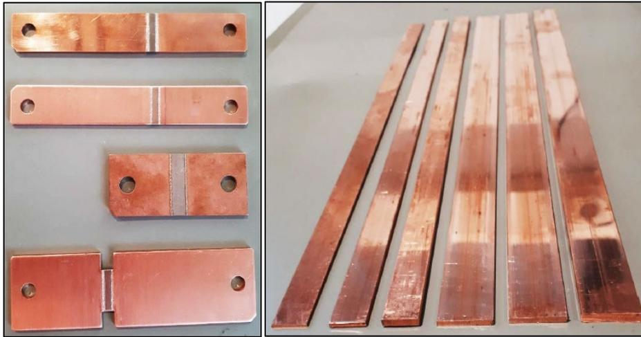
**Figure 21:** Shunts A to D from top to bottom (on the left) and busbars 1 to 6 (on the right) [29]
